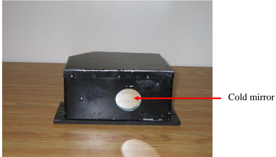
Figure 4 The laser device based on triangulation method.
