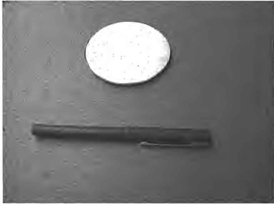
Figure 6.11 Microwave lens manufactured using glass epoxy
