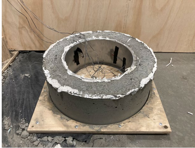
Figure 6. Single ring test. Source: Tanner Research Group.
