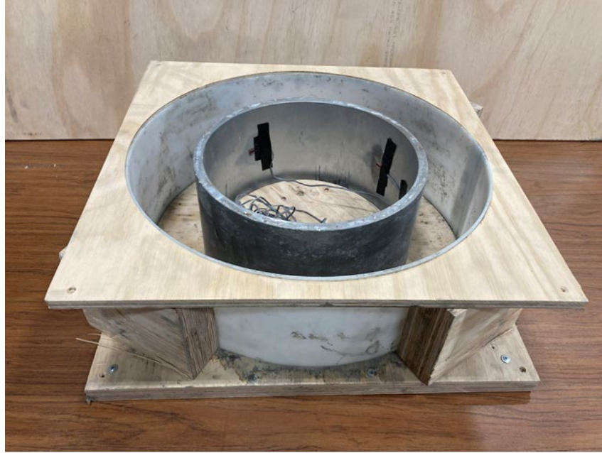
Figure 9. Single-ring setup. Source: Tanner Research Group.
