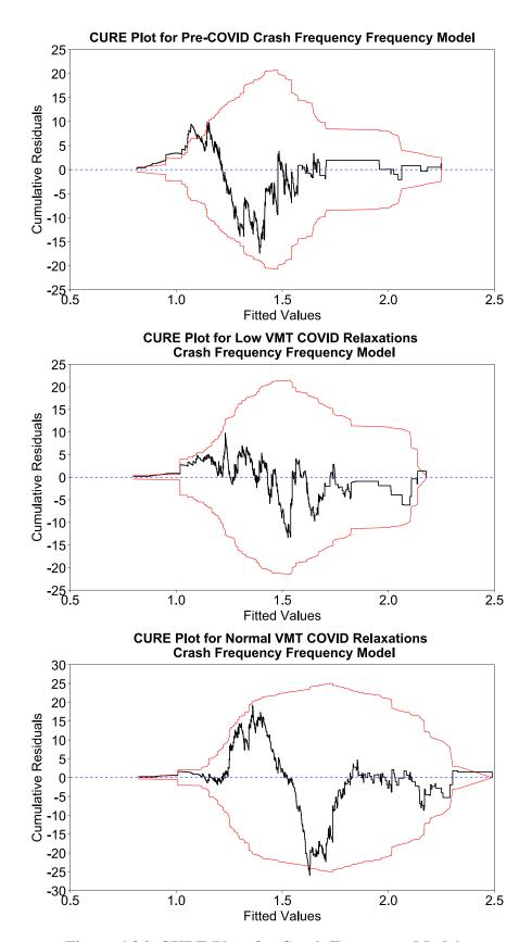
Figure 4.26: CURE Plots for Crash Frequency Models
