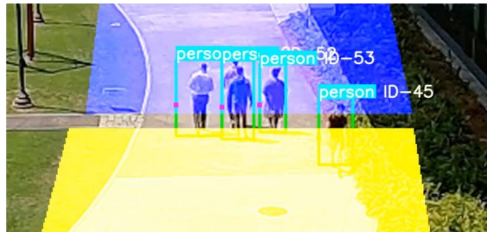
Figure 6 Sample of upscaled ROI of a frame, where five pedestrians are detected moving upwards (yellow to blue polygon)
