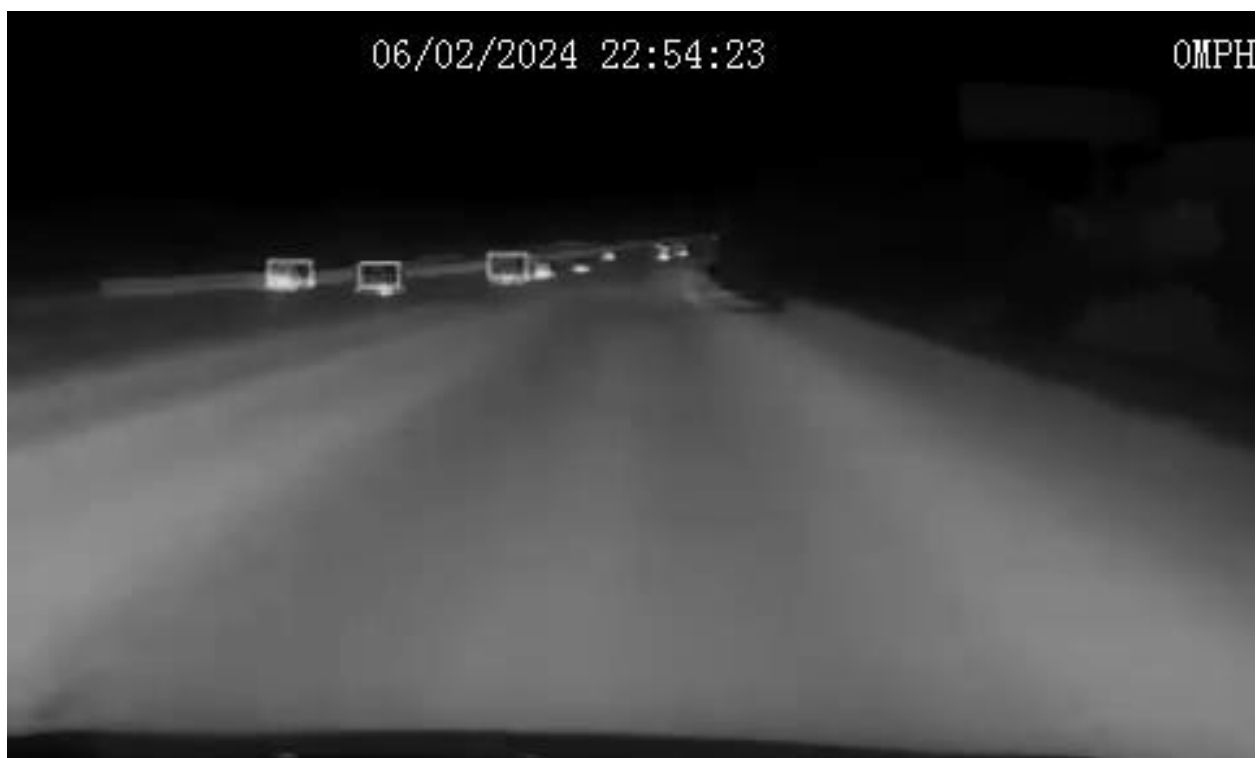
Figure 5.26: InfiRay sample frame in fog at night with multiple vehicles on the road
