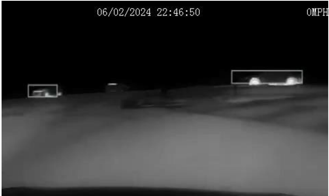
Figure 5.24: InfiRay sample frame in fog at night
