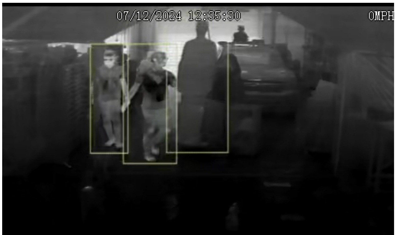
Figure 5.32: InfiRay sample frame with dense artificial fog
