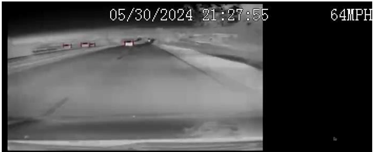
Figure 5.8: FLIR sample frame at night with night vision on
