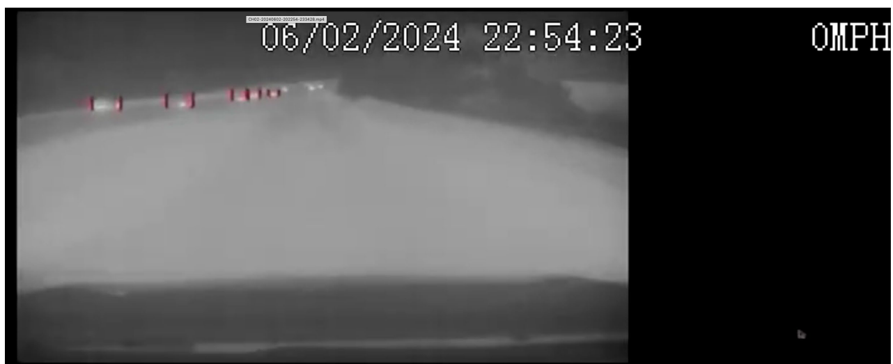
Figure 5.23: FLIR sample frame in fog at night with multiple vehicles on the road
