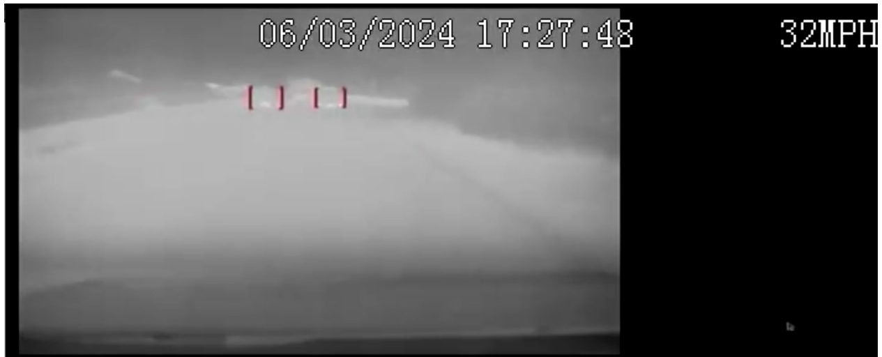
Figure 5.15: FLIR sample frame during daytime fog at low speed
