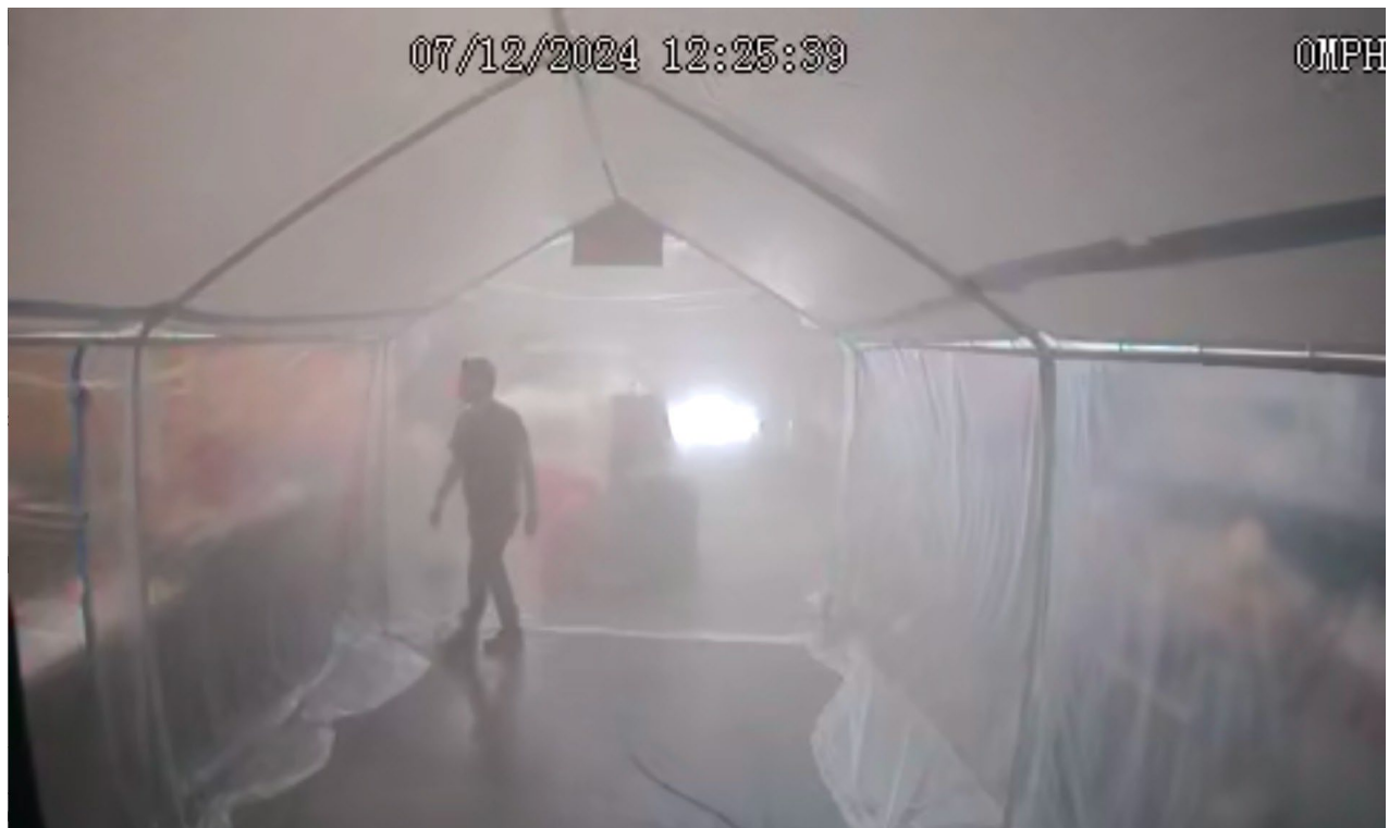
Figure 5.27: Sample frame from CAM-720 with light artificial fog
