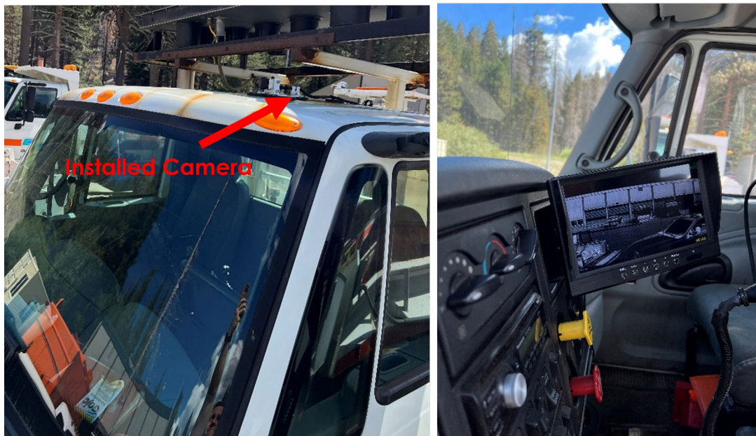
Figure 2.1: Installed IR cameras on a Caltrans vehicle
