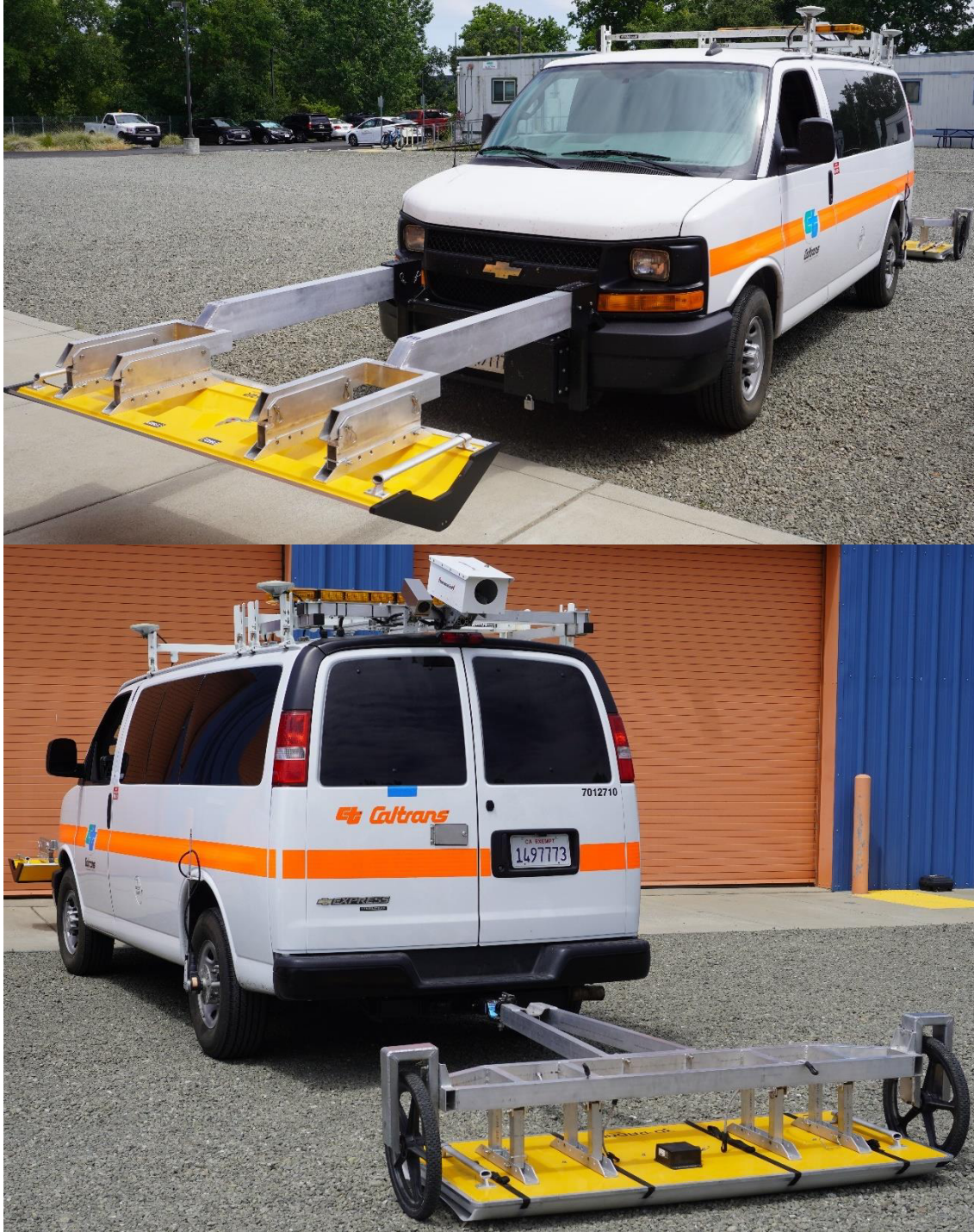
Figure 1.1: The Caltrans NDE vehicle (front and rear view). In project deployment, either the front or rear GPR antenna is used. The IR and B/W housing is mounted at the NDE vehicle rear on top of the roof.
