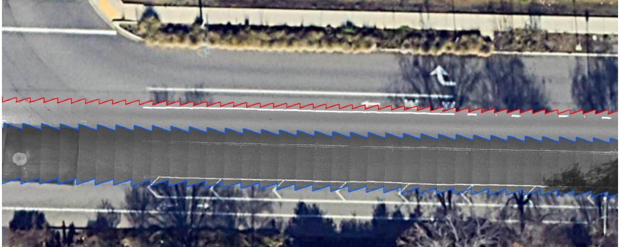
Figure 3.14: Second example overlay of mosaics from eastbound and westbound Hutchison Drive capture sessions. The result shows good alignment with the Google Earth satellite imagery as well as good run-to-run alignment. The mosaic with red outline is composed of images collected traveling westbound. The mosaic with blue outline is composed of images collected traveling eastbound.
