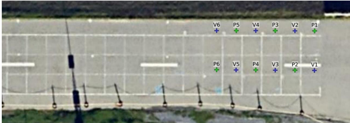
Figure 3.10: Surveyed ground control points overlay on Google Earth satellite image. The mismatch of the control points positions and the Google satellite image, approximately 0.5 meter in Northing and Easting direction, are within the error margin of the satellite image accuracy.
