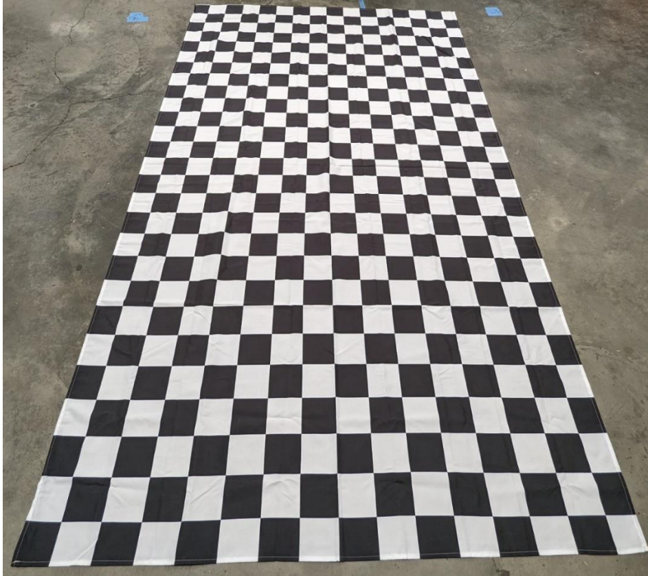
Figure 2.2: Checkered cloth laid on the ground for IR camera rectification calibration
