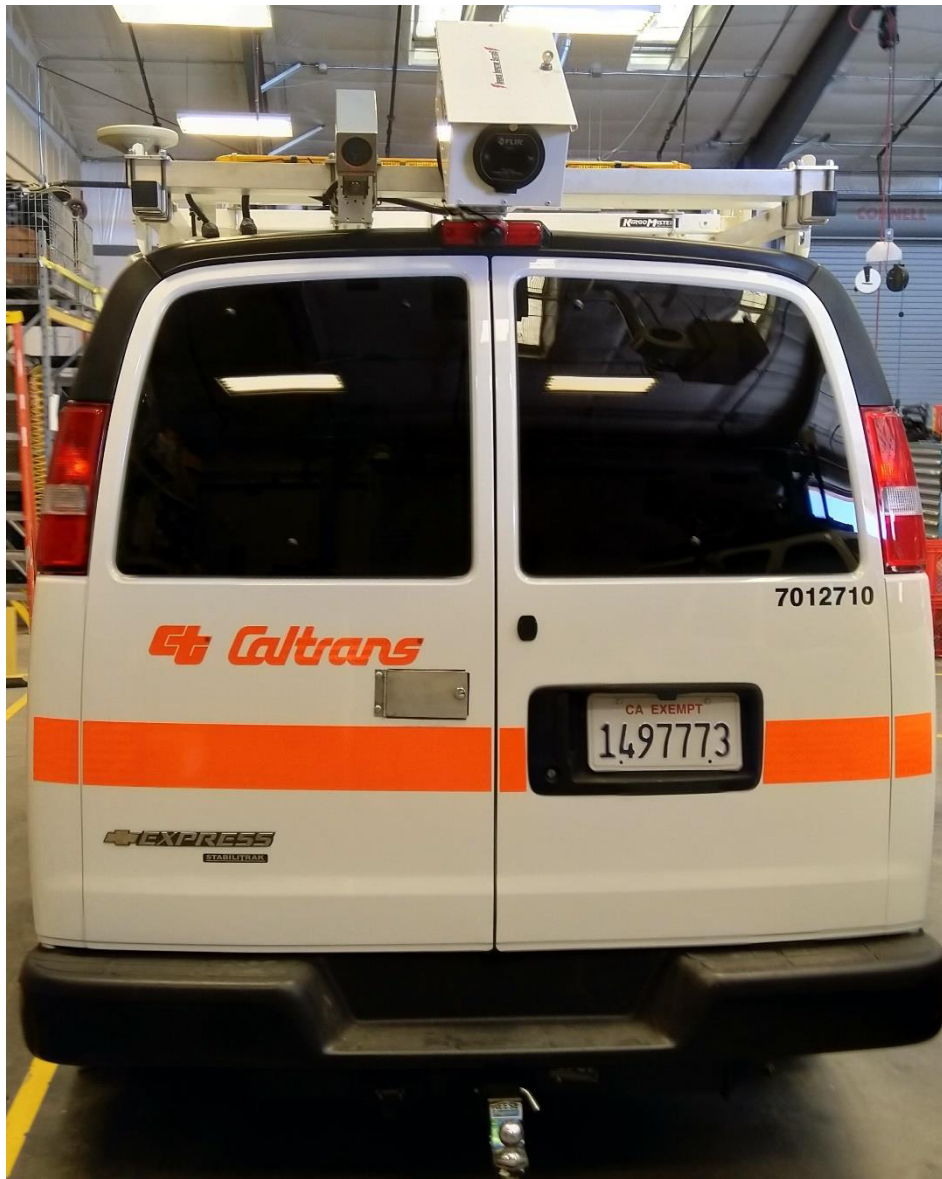
Figure 1.2: Caltrans NDE vehicle camera mounts (rear view). The large white box at the top center is the IR camera housing. The smaller silver box is the B/W housing.
