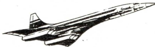
BAC-SUD-AVIATION CONCORDE Anglo-French supersonic 132 passenger transport has ogive, high lift, wing and pivoting nose for takeoff and landing. Speed 1,450 m.p.h. (Mach 2.2) at cruise altitude of 62,000 feet; range 4,155 miles; four 38,300-lbs.t. with reheat turbojets.
