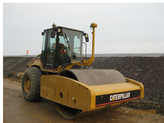
Intelligent compaction roller mapping on subgrade layer on SR-22 project in Pennsylvania (September 20, 2009)
