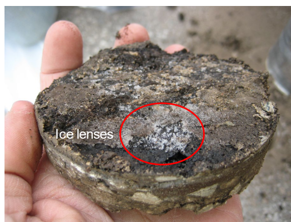
Ice lenses within the pavement inter layers
