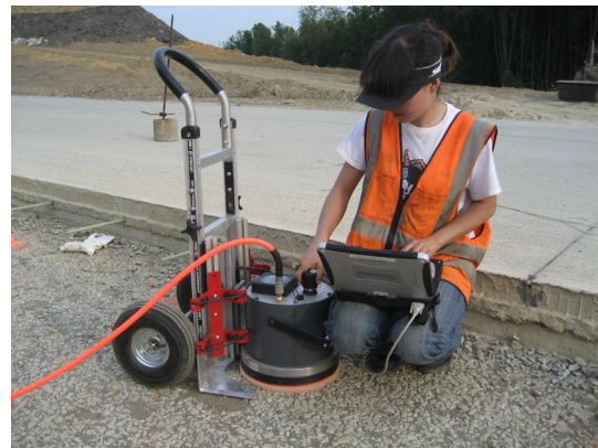
Air permeability testing on cement treated base layer on SR-22 project in Pennsylvania (September 17, 2009)
