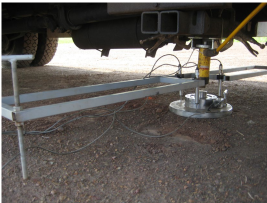
304.8 mm diameter static plate load test setup on compacted subgrade on US 10 project in Wisconsin (May 25, 2010)
