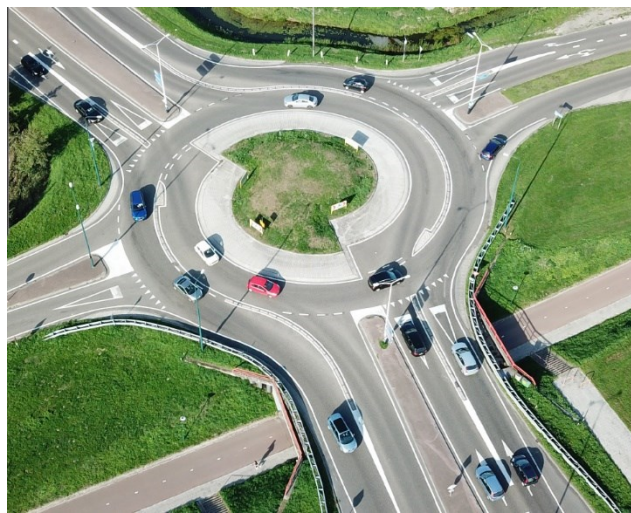
Figure 4-2 Turbo Roundabout, Delft. (Turbo Roundabout, n.d.)
