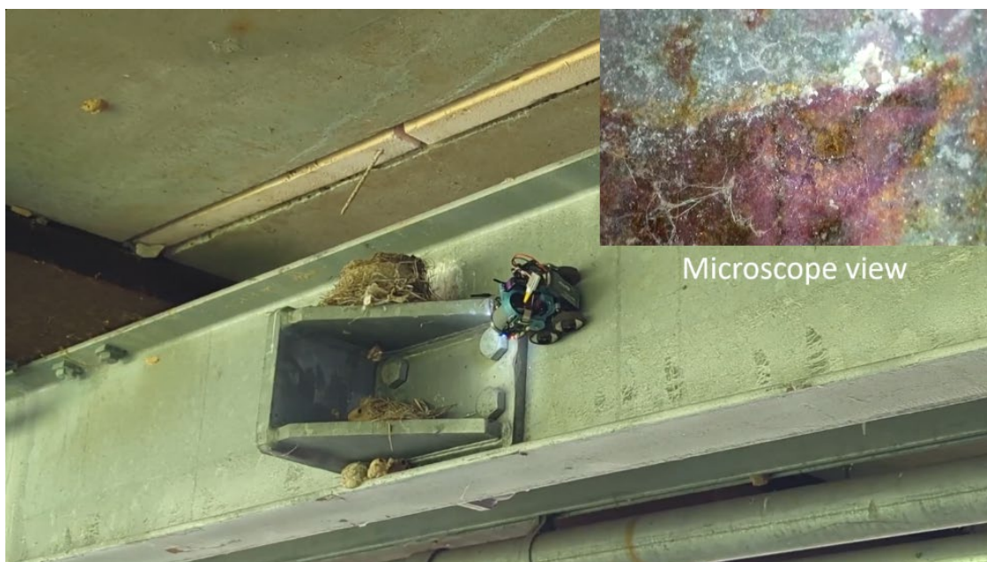
Figure 94. Crawler Access to a Potentially Corroded Area via Microscopic View
