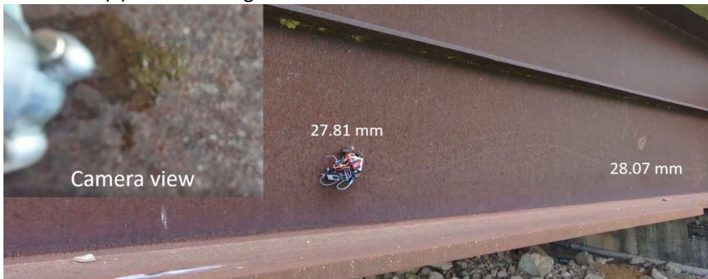
(b) Web thickness measurements and readings at two designated points
