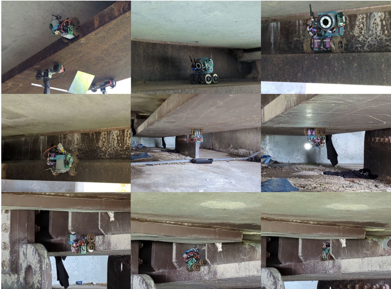
Figure 93. Crawler Access to Narrow Spaces for Weld Connection Inspection
