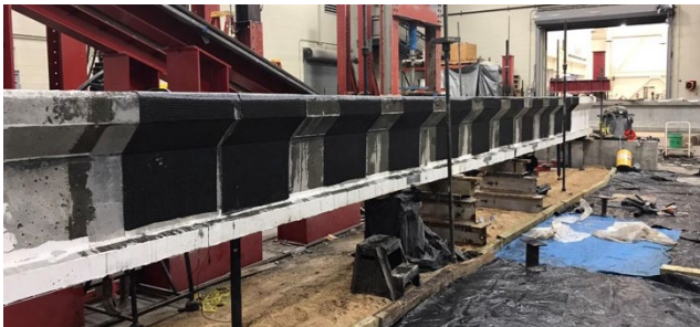
Figure 1: Impact testing and repair using CFRP
