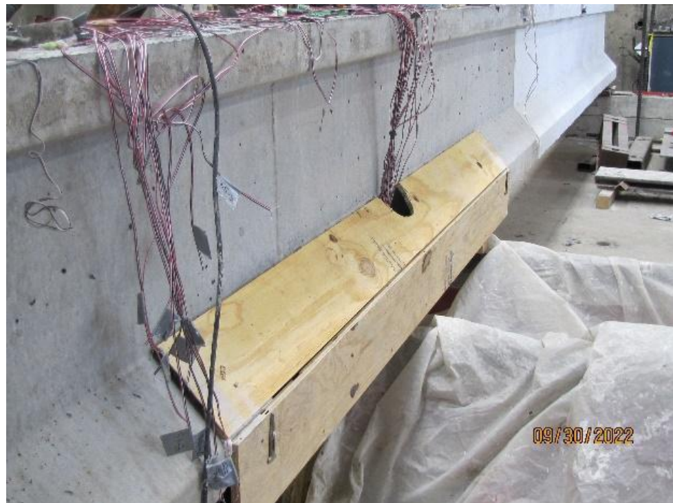
Figure G-11. Splicing and formwork of the spliced 25% (Girder G11)
