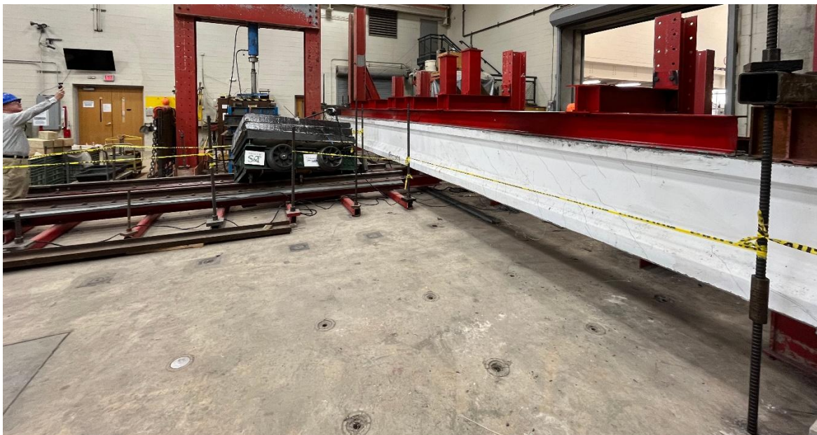
Figure C-40. Cracking of the girder after impact
