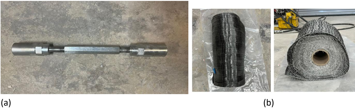
Figure 6-1. Methods used for structural repair (a) Mechanical strand splicing (b) CFRP composite
