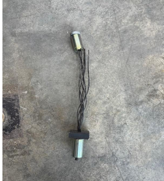
Failure of seven-wire prestressing strand specimen after tensile testing.
