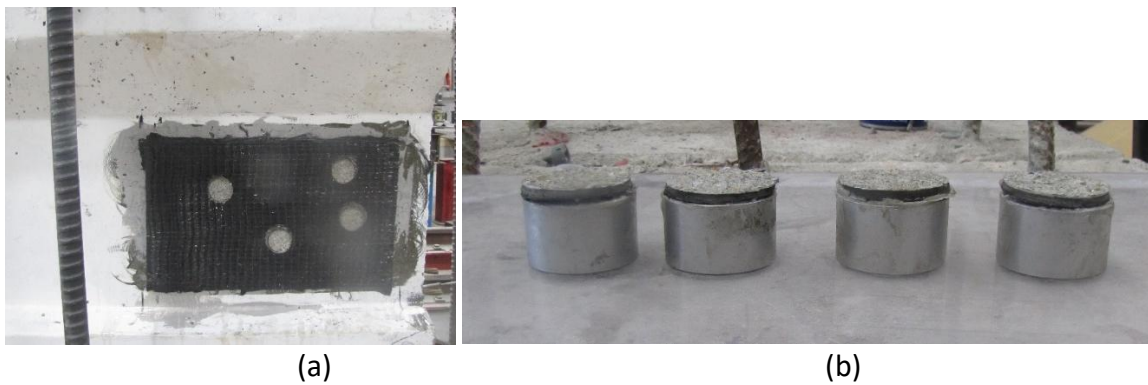
Figure 6-23. (a) Witness panel for pull-off test, (b) Pull-off test specimens' failure
