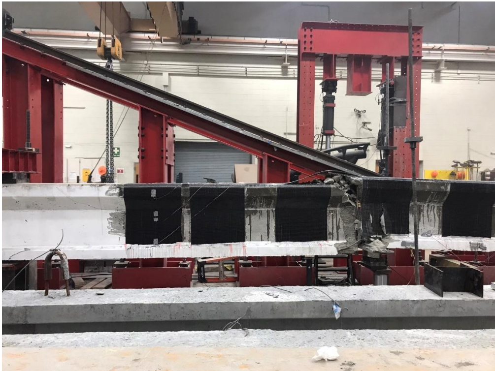
Figure G-20. Girder deflection and failure
