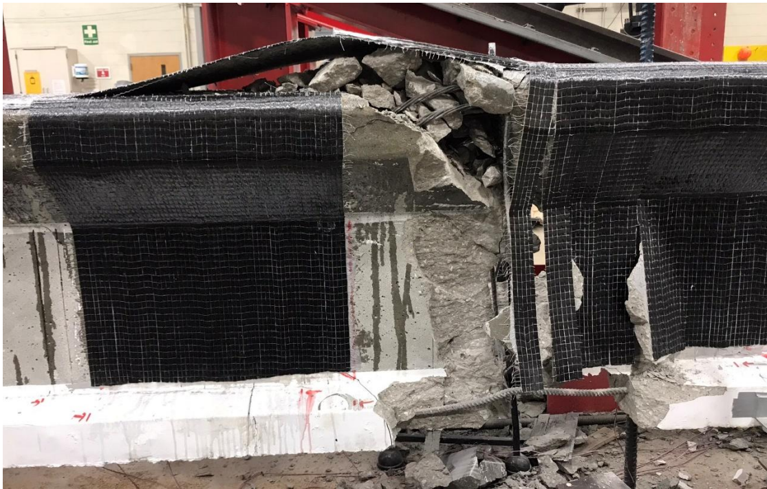
Figure G-21. Rupture of CFRP longitudinal plies
