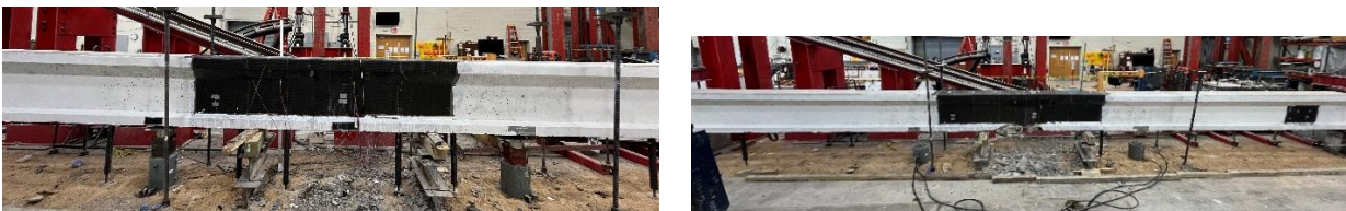
Figure G-30. Hybrid girder testing after CFRP installation
