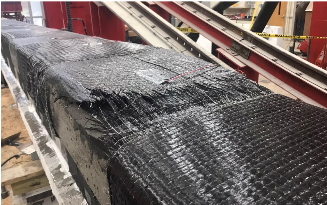
Figure G-25. Testing and failure of the repaired girder
