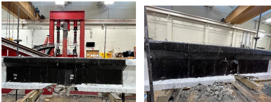
Figure G-31. Rupture and delamination of CFRP
