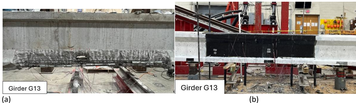
Figure 6-29. (a) Girder being repaired with mechanical strand splice, (b) Photograph of completely repaired girder (hybrid system) with CFRP U-wraps as confinement
