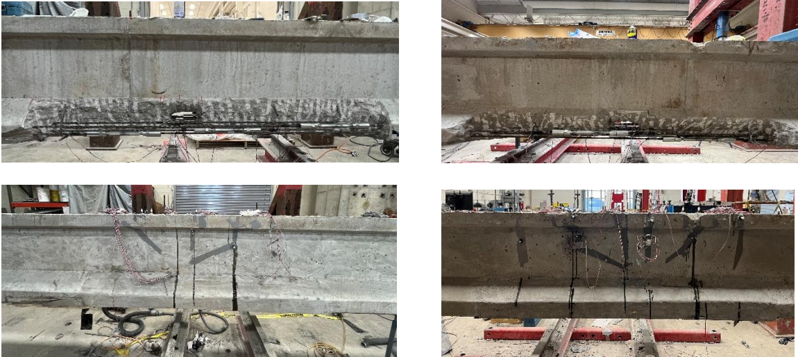
Figure G-29. Strand repair and grout patching
