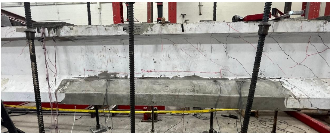
Figure G-14. Formwork and casting grout of the patched area
