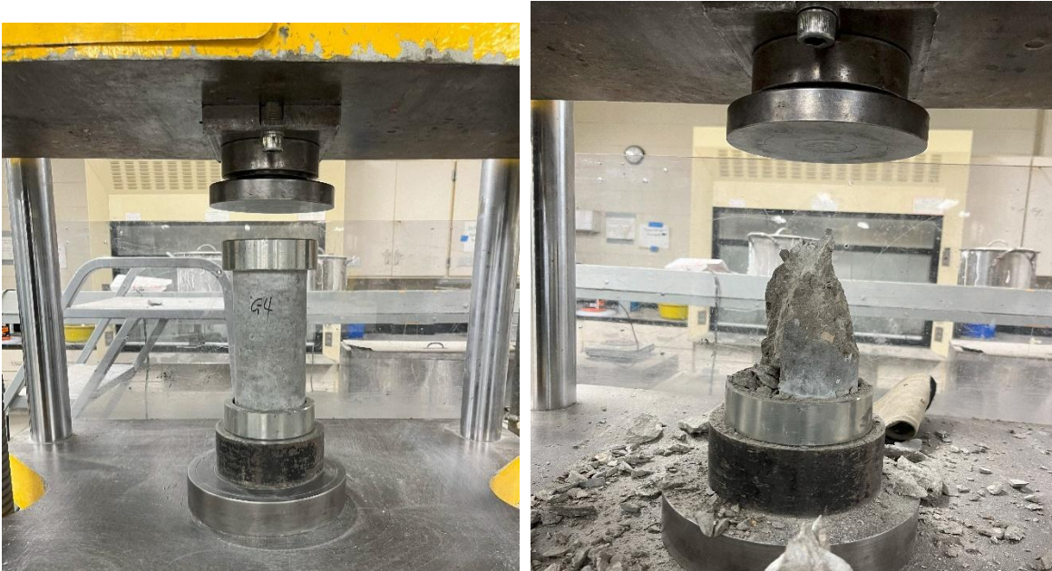
Figure D-31. Compression standard cylinder test (a) Compression testing configuration of a 4x8 inch cylindrical specimen under uniaxial loading (b) Failure of specimen
