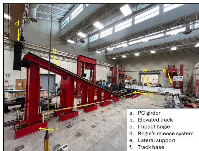
Figure 1-1. Impact simulator test setup
