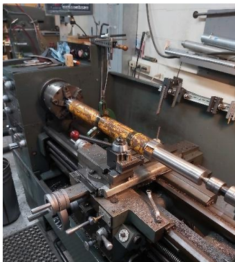
Figure B-30. Impact bogie fabrication (a) Axle bearing plate, (b) Bogie main frame, (c) Machining the bogie wheels, (d) Machining the axle, (e) Bogie and wheels assembly
