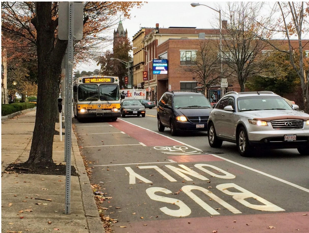
TTLs typically expand parking lanes, making room for bike lanes and giving cyclists a new buffer between parked cars and moving vehicles. Photo courtesy of City of Everett, MA.
