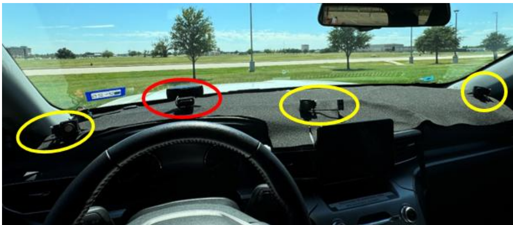
Figure 11. Smart Eye Camera Setup on Vehicle Dashboard.
