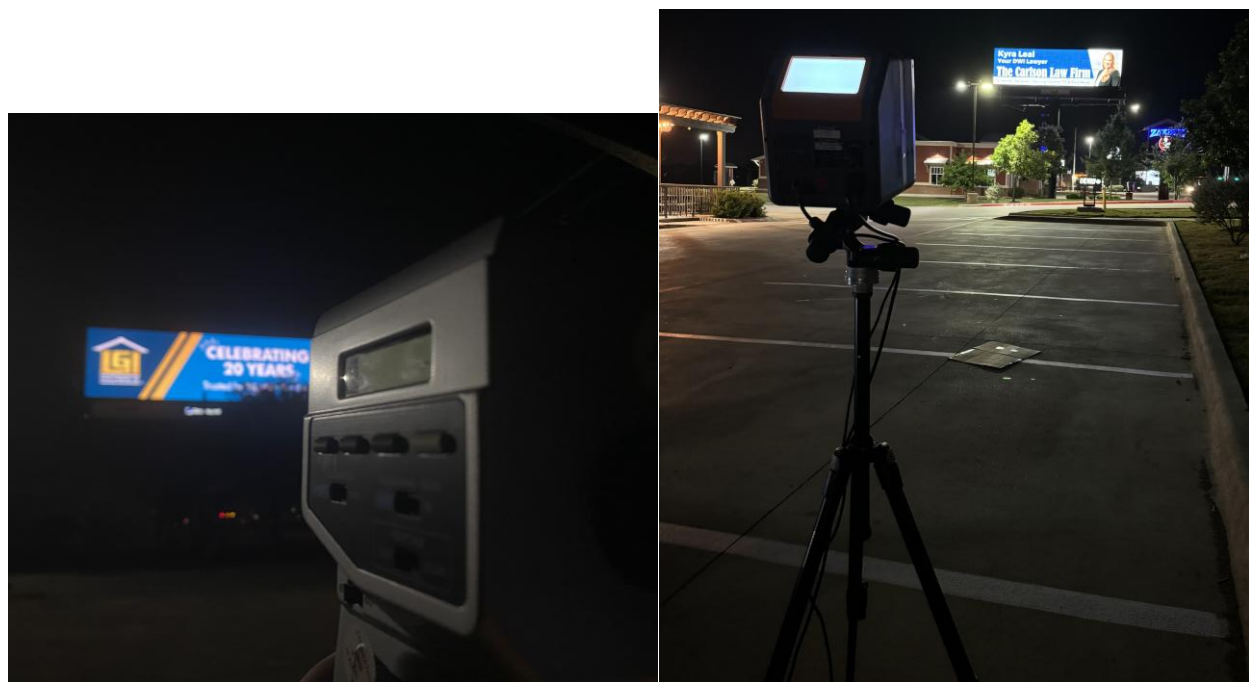
Figure 13. Handheld Luminance Meter (Left) and Imaging Colorimeter (Right).
