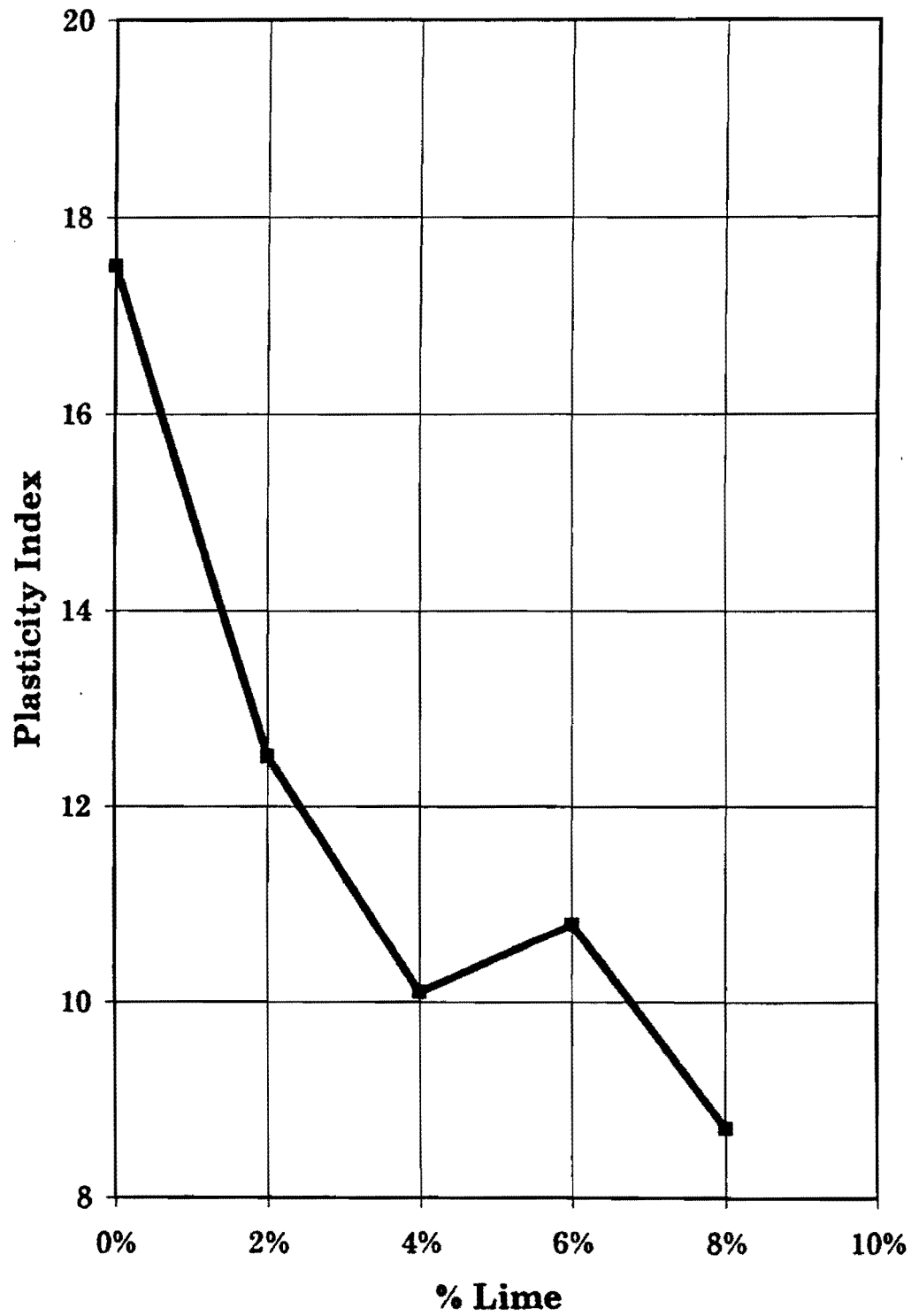
Figure 4.15: PI Versus Lime Percentages to Verify the Optimum Lime Content at 4%.
