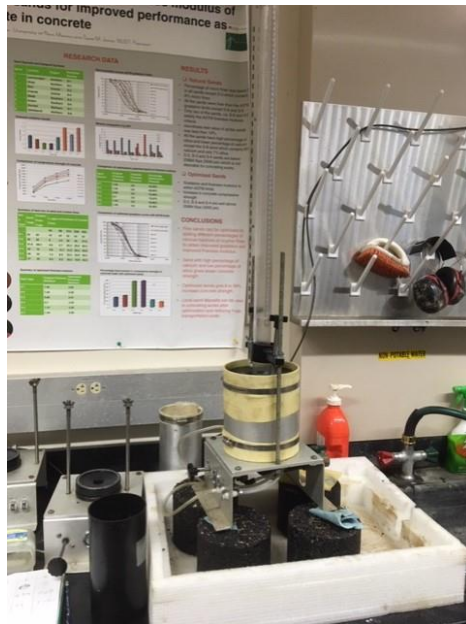
FIGURE 35 Permeability test setup
