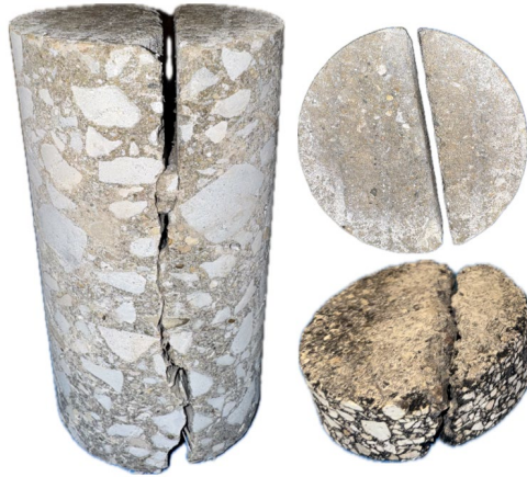
Figure 103. Photo. Test No. 5: side, top and bottom views of core extracted from I-72 EB at station 15+16 at the middle of a transverse joint without a longitudinal crack.
