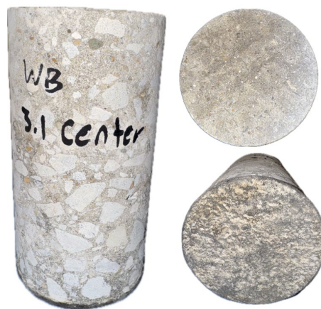
Figure 117. Photo. Test No. 5: side, top and bottom views of core extracted from I-72 WB at station 109+78 at the slab center.
