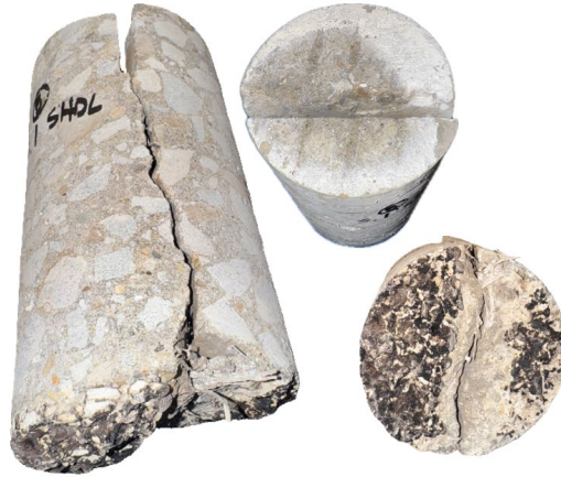
Figure 106. Photo. Test No. 8: side, top and bottom views of core extracted from I-72 EB at station 144+43 at the lane—shoulder joint.
