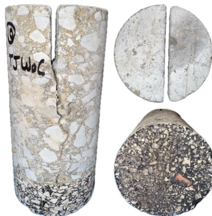
Figure 105. Photo. Test No. 7: side, top and bottom views of core extracted from I-72 EB at station 82+66 at the middle of a transverse joint without a longitudinal crack.
