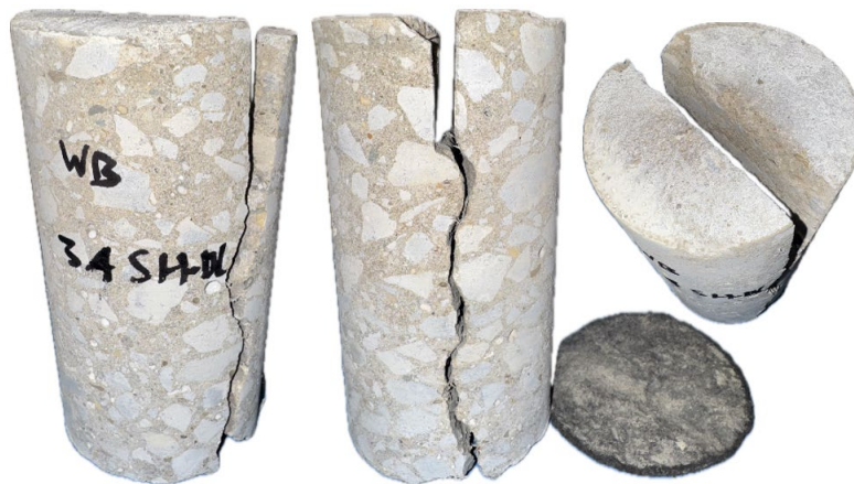
Figure 120. Photo. Test No. 8: sides, top and NWGF views of core extracted from I-72 WB at station 109+43 at the lane—shoulder joint.
