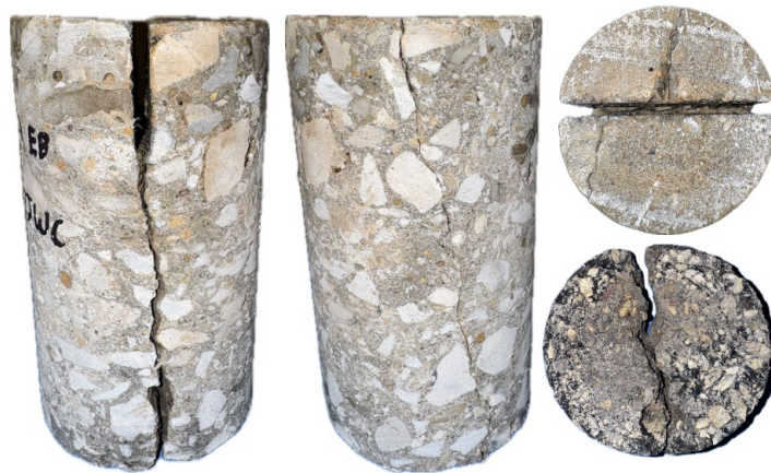
Figure 101. Photo. Test No. 3: sides, top and bottom views of core extracted from I-72 EB at station 15+04 at the middle of a transverse joint with a longitudinal crack.
