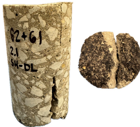
Figure 104. Photo. Test No. 6: side, and bottom views of core extracted from I-72 EB at station 82+61 at the lane—shoulder joint.
