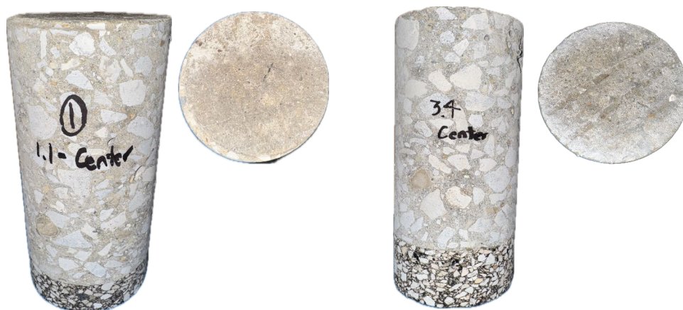
Figure 62. Photo. Side and top view of cores extracted from slab centers.
