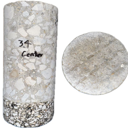
Figure 109. Photo. Test No. 11: side and top views of core extracted from I-72 EB at station 144+63 at the slab center.
