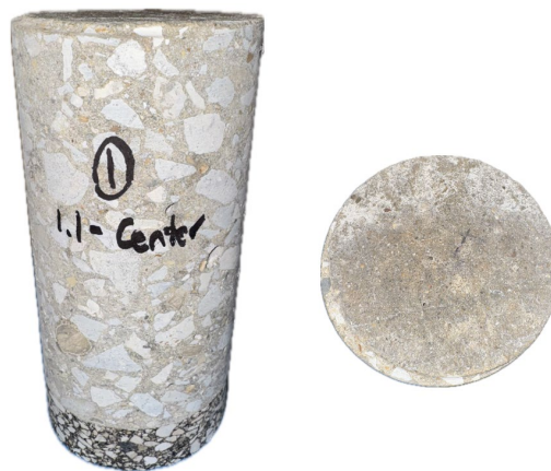
Figure 99. Photo. Test No. 1: side and top views of core extracted from I-72 EB at station 14+77 at the slab center.
