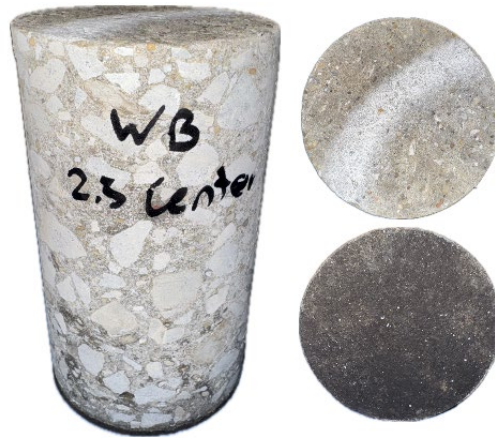
Figure 115. Photo. Test No. 3: side, top and bottom views of core extracted from I-72 WB at station 150+82 at the slab center.
