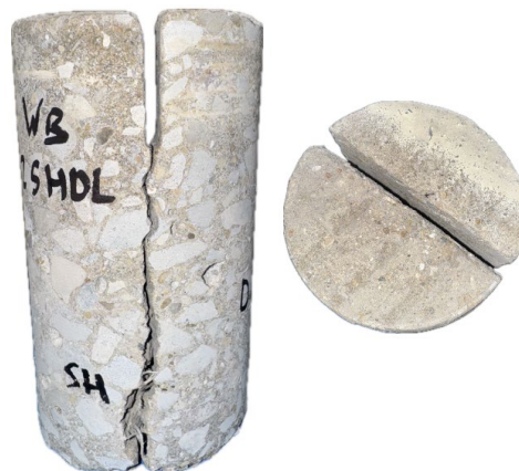
Figure 114. Photo. Test No. 2: side and top views of core extracted from I-72 WB at station 150+59 at the lane—shoulder joint.
