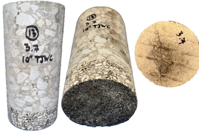
Figure 112. Photo. Test No. 14: side, bottom and top views of core extracted from I-72 EB at station 144+71 at 10" from a transverse joint with a longitudinal crack (on crack path).
