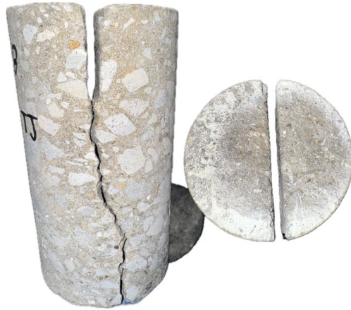
Figure 118. Photo. Test No. 6: side, and top views of core extracted from I-72 WB at station 109+66 at the middle of a transverse joint.
