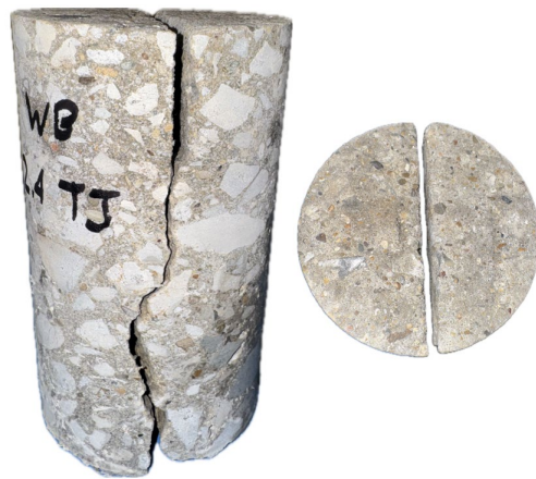
Figure 116. Photo. Test No. 4: side, and top views of core extracted from I-72 WB at station 150+58 at the middle of a transverse joint.
