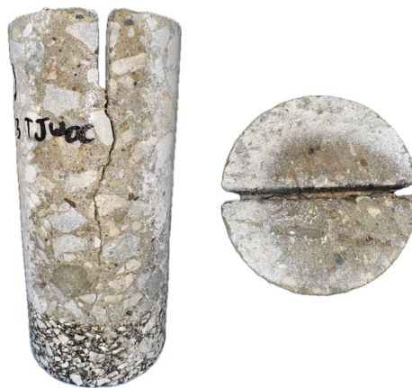
Figure 108. Photo. Test No. 10: side and top views of core extracted from I-72 EB at station 144+54 at the middle of a transverse joint without a longitudinal crack.
