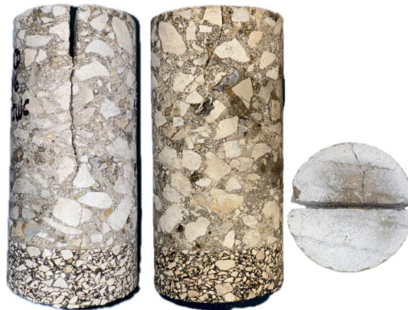
Figure 111. Photo. Test No. 13: sides, and top views of core extracted from I-72 EB at station 144+72 at the middle of a transverse joint with a longitudinal crack.
