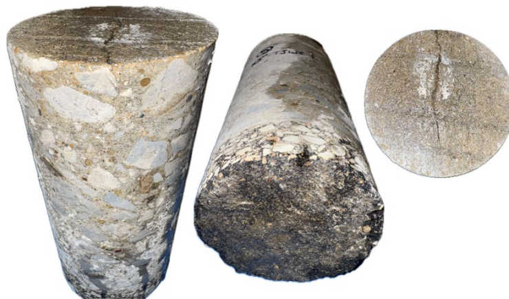
Figure 102. Photo. Test No. 4: side, bottom and top views of core extracted from I-72 EB at station 15+03 at 10" from a transverse joint with a longitudinal crack (on crack path).
