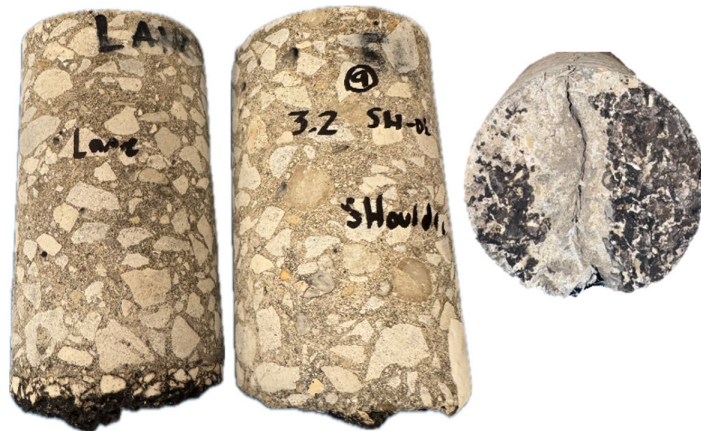
Figure 107. Photo. Test No. 9: sides and bottom views of core extracted from I-72 EB at station 144+55 at the lane—shoulder joint.
