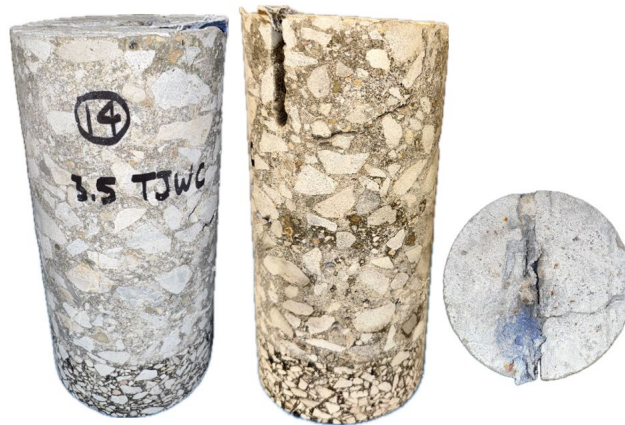
Figure 110. Photo. Test No. 12: sides, and top views of core extracted from I-72 EB at station 144+78 at the middle of a transverse joint with a longitudinal crack.
