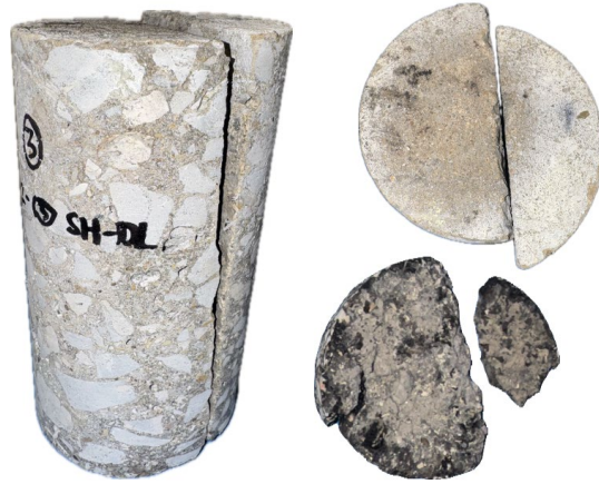
Figure 100. Photo. Test No. 2: side, top and bottom views of core extracted from I-72 EB at station 14+93 at the lane—shoulder joint.
