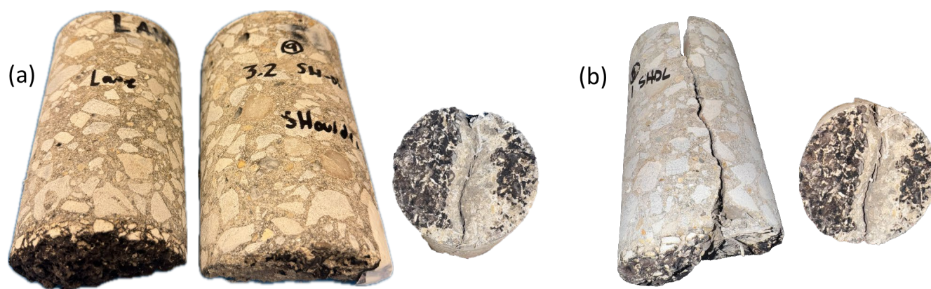
Figure 66. Photo. Example of cores extracted from driving lane-shoulder longitudinal joints showing full-depth joint activation and an advanced HMA interlayer degradation. (a) Core split along longitudinal joint. (b) Core that remained held together by only a few macrofibers.
