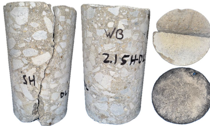
Figure 113. Photo. Test No. 1: sides, top and bottom views of core extracted from I-72 WB at station 150+68 at the lane—shoulder joint.
