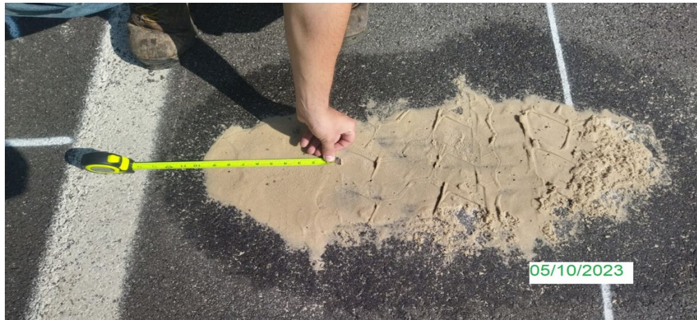
Figure 53 Example of sand patch used to measure truck tire offset.
