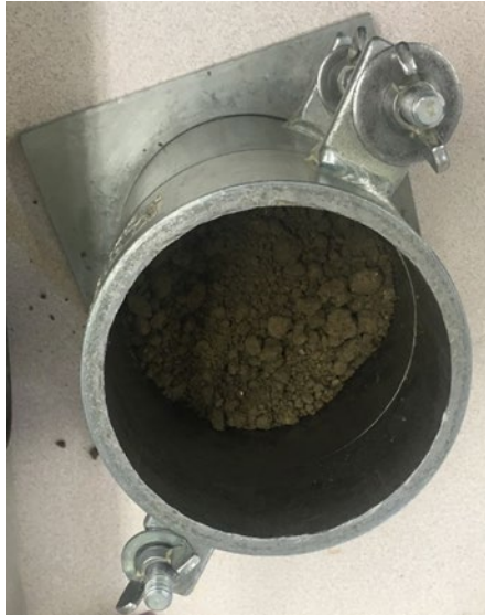
Figure 3.4 Layer of soil before being compacted
