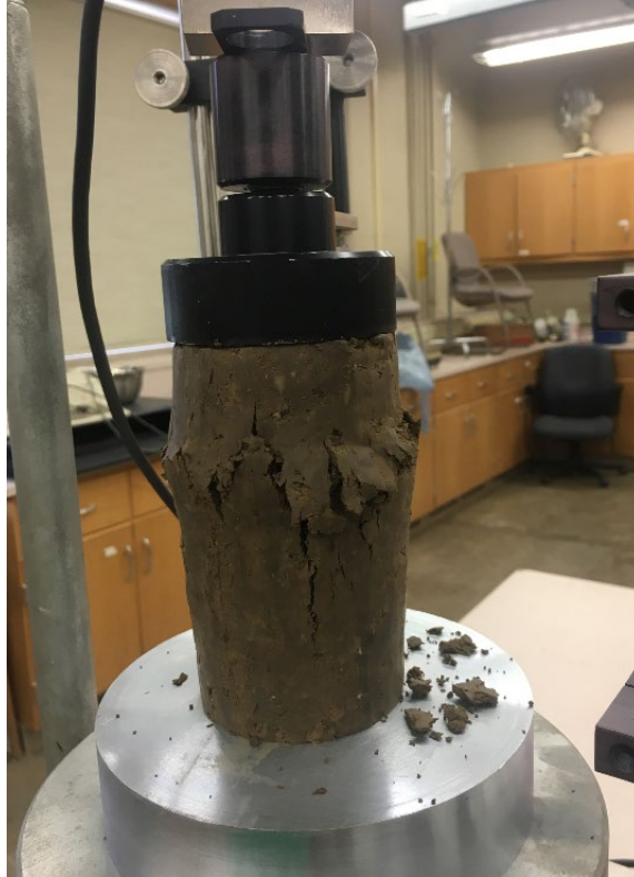
Figure 3.12 Soil specimen after failure
