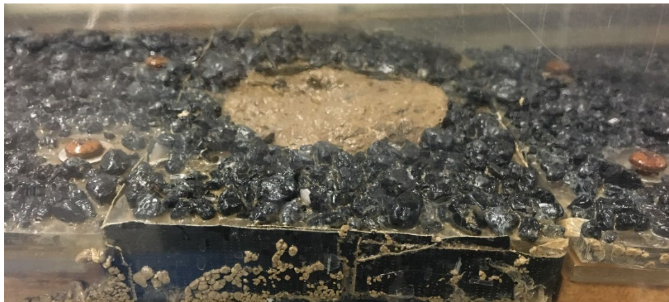
Figure 3.27 Example of soil specimen after being eroded
