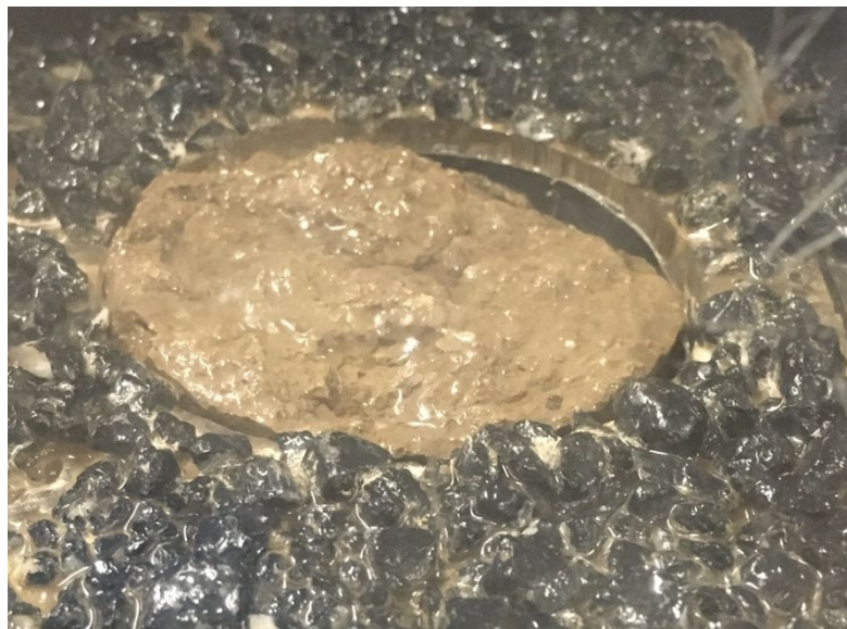
Figure 4.19 Final erosion depth after about 5 hours
