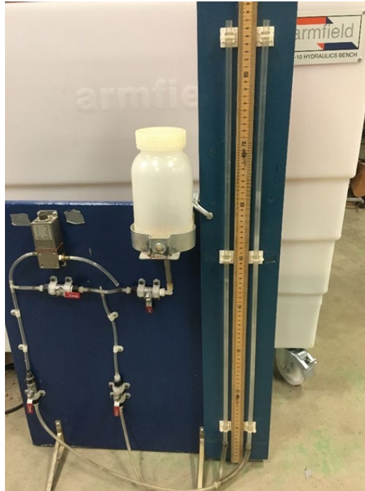
Figure A.3 Static manometer setup
