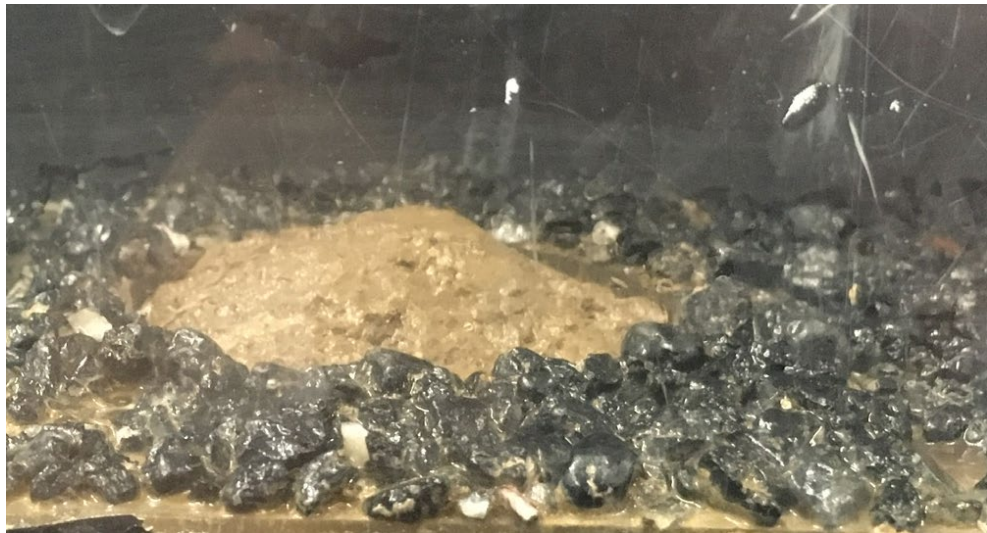
Figure 4.22 Example of cone-shaped erosion pattern
