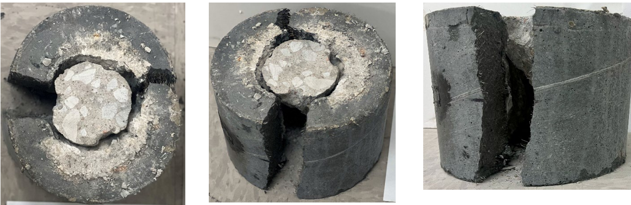
a) Failure mode of specimen CC6-UHPC2#1
