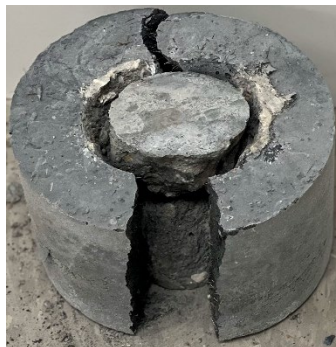
e) Failure mode of specimen CC7.5-UHPC2#2
