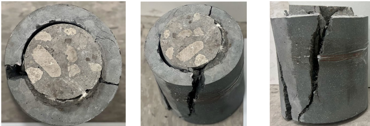
d) Failure mode of specimen CC7.5-UHPC1#1
