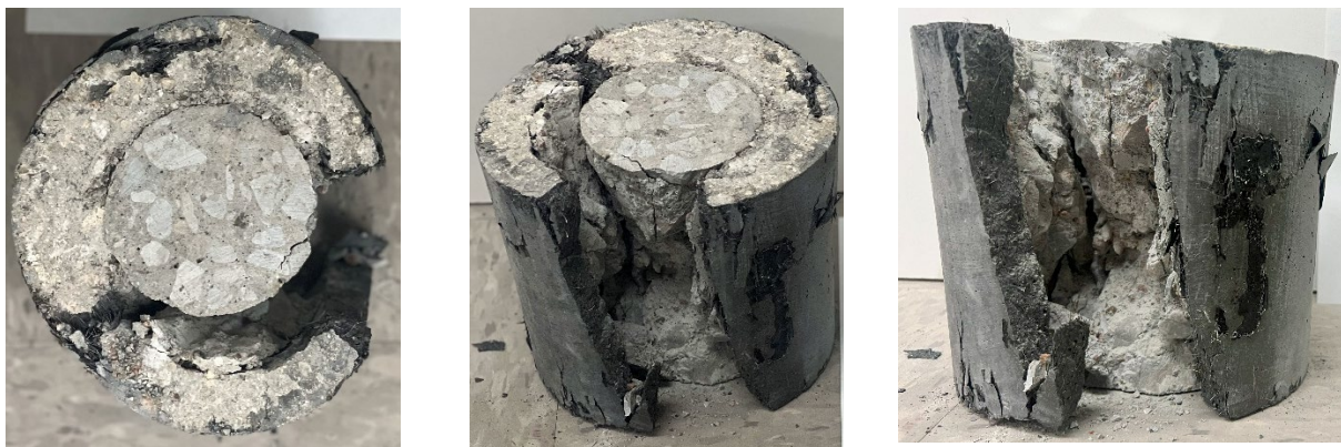
b) Failure mode of specimen CC6-UHPC1#2
