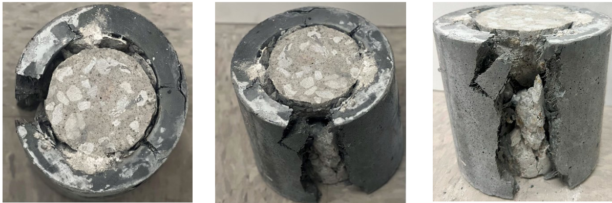
a) Failure mode of specimen CC6-UHPC1#1
