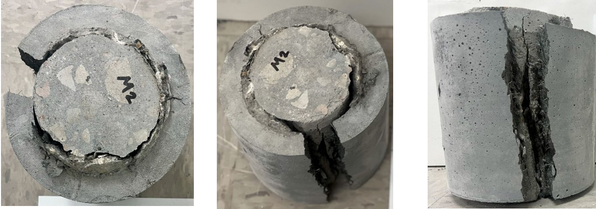
f) Failure mode of specimen CC7.5-UHPC1#3
