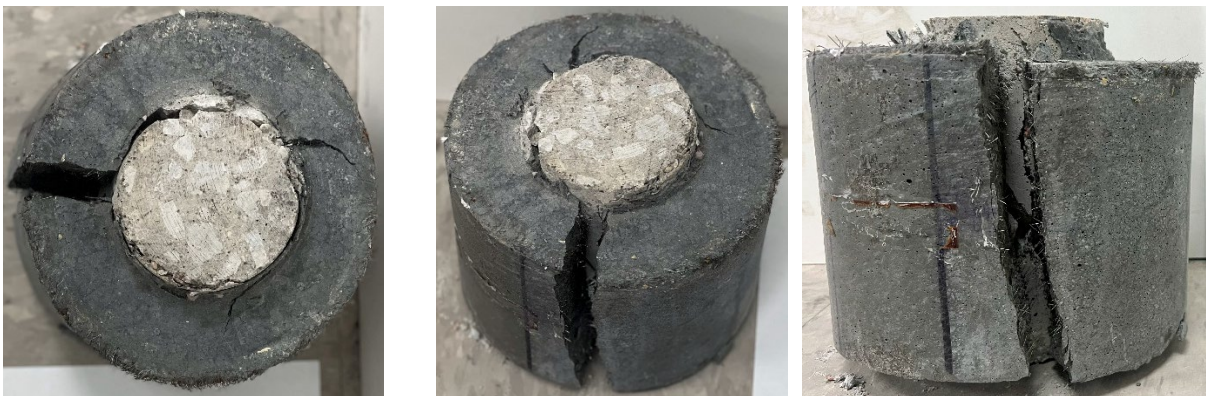
b) Failure mode of specimen CC6-UHPC2#2
