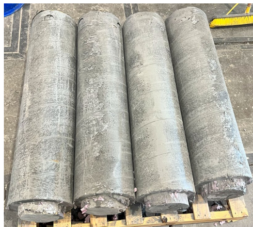
Figure 4.2 Samples of the full-scale compression members encased with UHPC
