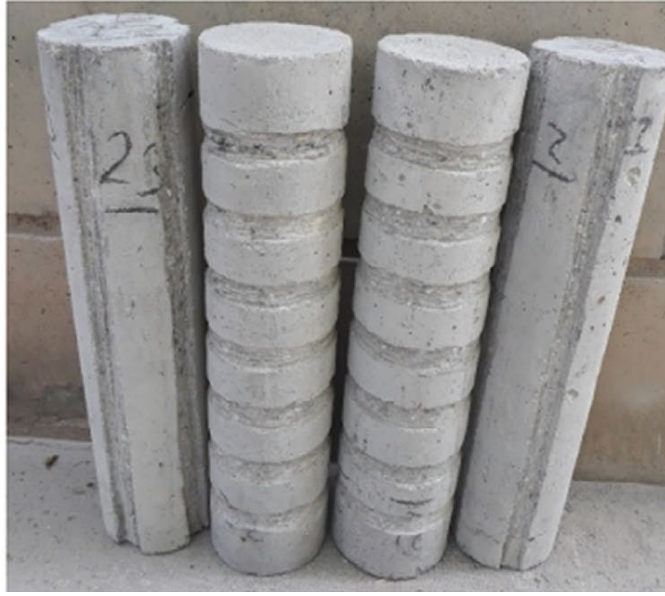
Figure 2.13 Horizontal and longitudinal grooves (Dadvar et al., 2020)
