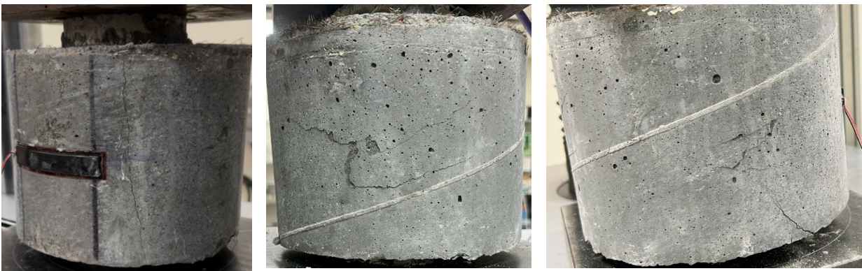
Figure 4.29 Cracks initiation in specimens during testing
