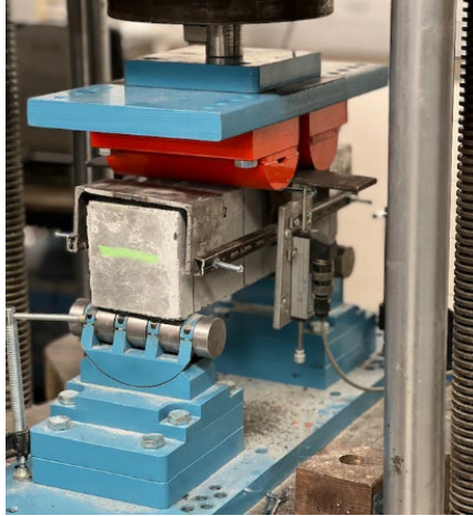
Figure 4.5 Flexural testing of UHPC prism
