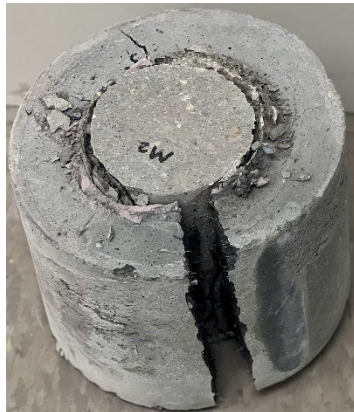
d) Failure mode of specimen CC7.5-UHPC2#1
