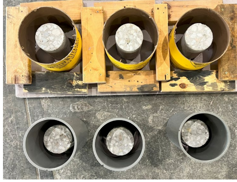
Figure 4.17 Formwork for the first phase specimens
