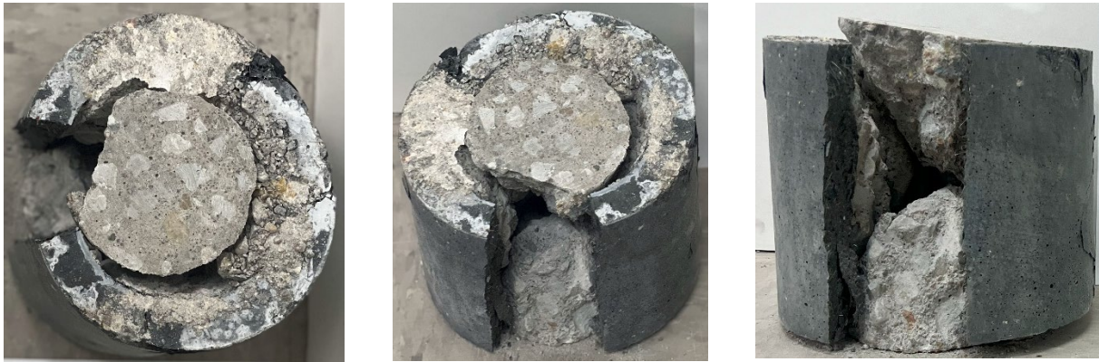
c) Failure mode of specimen CC6-UHPC1#3
