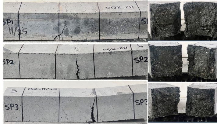
Figure 4.8 Tested flexural prisms after failure.
