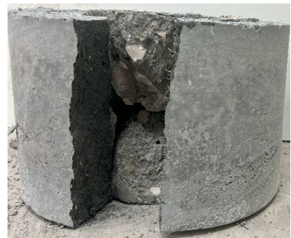
e) Failure mode of specimen CC7.5-UHPC2#2
