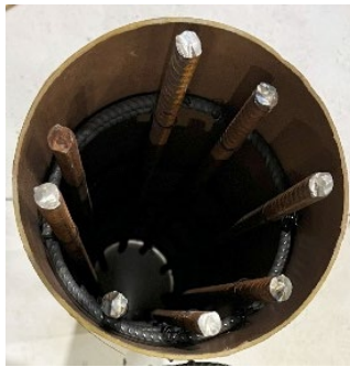
Figure 4.14 Specimen with surface sand blasted before cast CC
