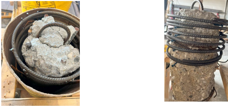
Figure 4.16 Top reinforcement of UHPC jacket
