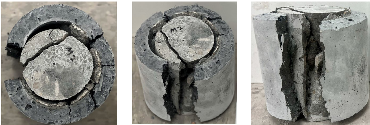
e) Failure mode of specimen CC7.5-UHPC1#2
