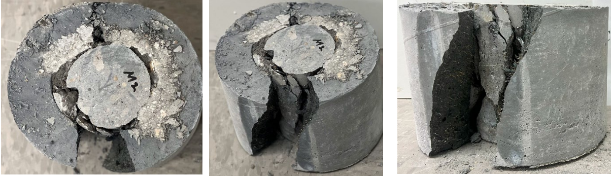
f) Failure mode of specimen CC7.5-UHPC2#3
