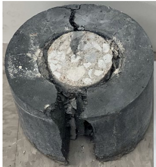
c) Failure mode of specimen CC6-UHPC2#3
