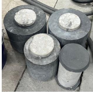
Figure 4.1 Samples of the small cylinders confined with UHPC
