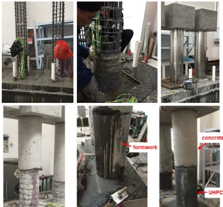
Figure 2.8 Construction of UHPC jacket (Wenting et al. 2022)
