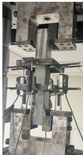
Figure 4.9 Direct tension testing of UHPC prism
