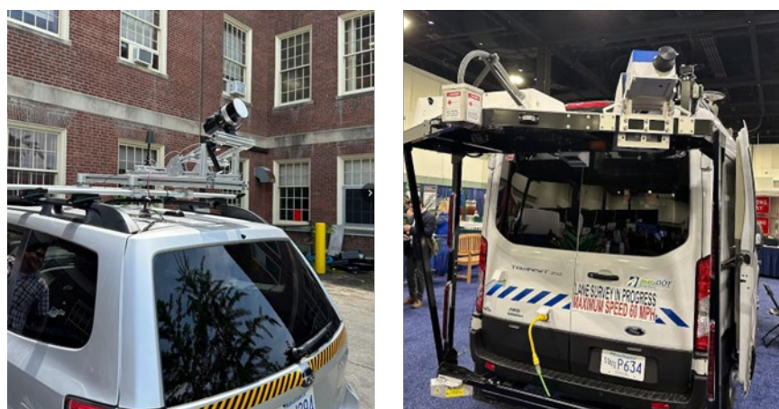
Figure 2.4: Integrated data collection vehicle with RESEPI (L) and Z+F (R) systems
