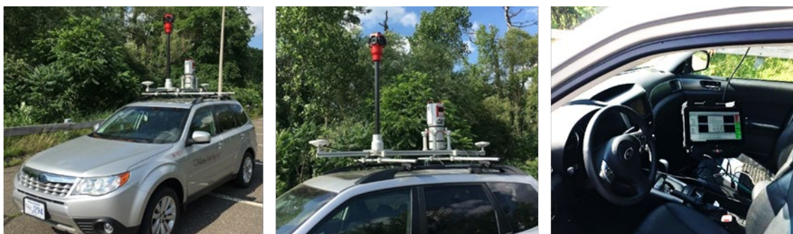
Figure 2.3: Integrated data collection vehicle with RIEGL system
