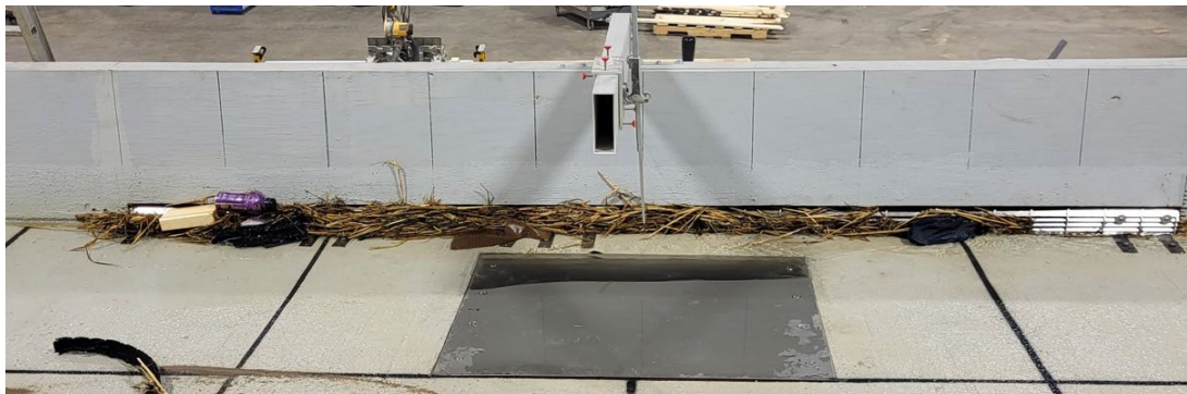
Figure 2: Full-scale physical model of barrier inlet with screen partially occluded in IIHR's hydraulics laboratory.
