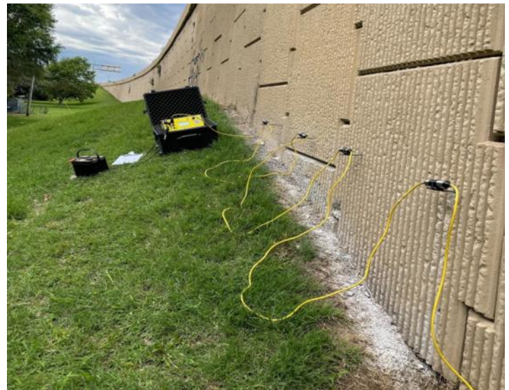
Field Electrical Resistivity Setup at the MSE Wall at US-54 over McLean Blvd. in Wichita, Kansas
