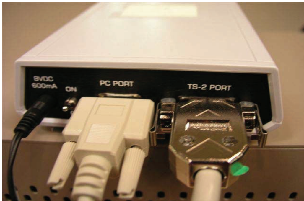
Figure 12. Connection of TS2 Cable and RS-232 Cable to the CID.
