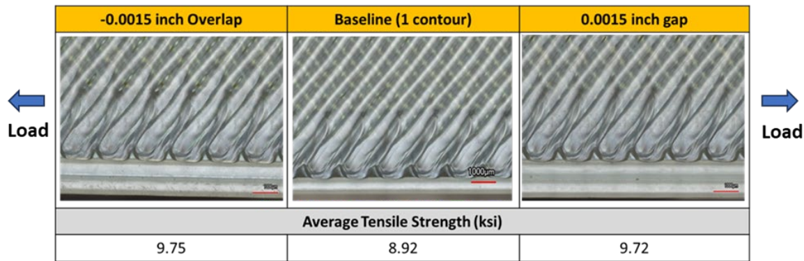
Figure 27. Microstructure comparison for XY specimens when CC2 setting is varied
