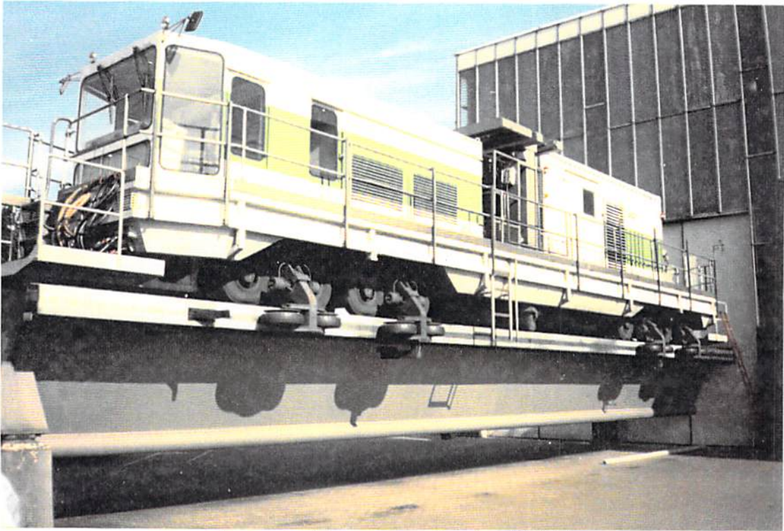
Figure 9. Emergency Towing Vehicle
