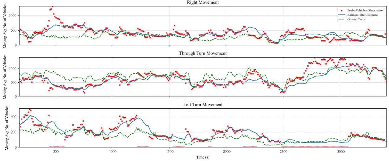
Figure 7: Comparison between Kalman filter-derived TM counts versus CV observations and ground truth counts for the EB approach at market penetration = 10%
