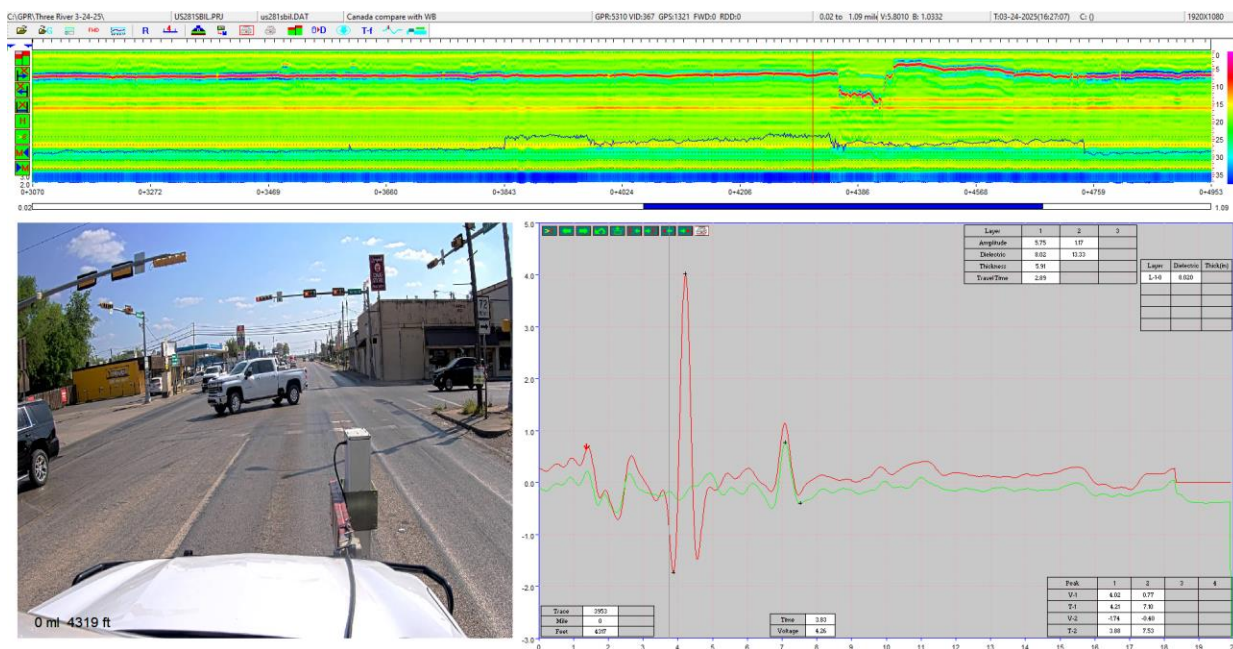
Figure 4-4 GPR used for mapping the layer thickness
