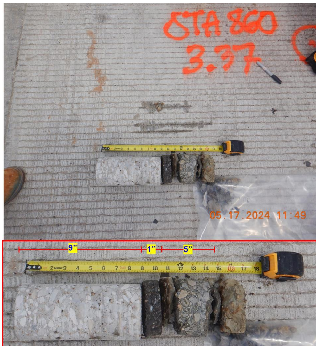
Figure 5-59 Inconsistency in Slab thickness as observed in Panola US59
