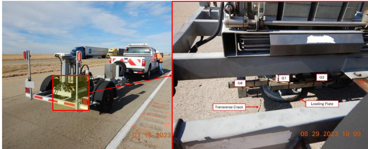
Figure 4-5 FWD, a trailer-mounted device
