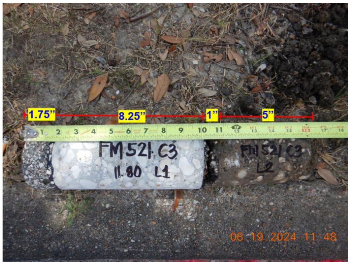
Figure 5-48 Concrete core taken in 12.26mils deflection
