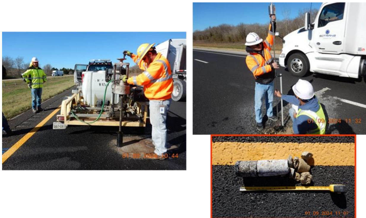
Figure 4-3 Coring operation with cored sample
