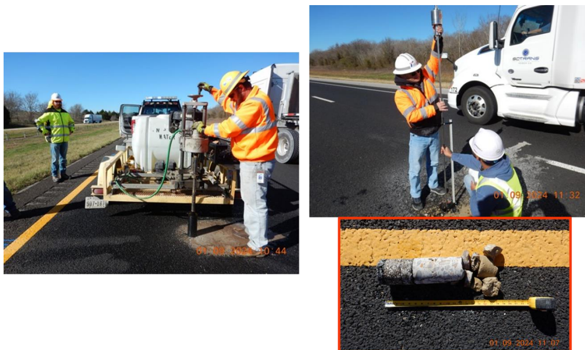
Figure 5-17 Coring and DCP test on the points of interest
