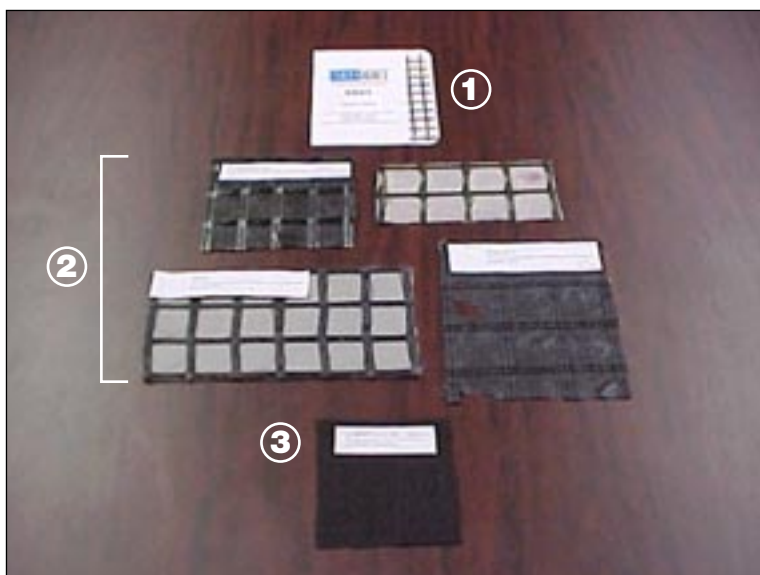
Figure 2. Different types of geosynthetics: 1) grid (protuding out of a paper envelope), 2) composites, 3) fabric.
