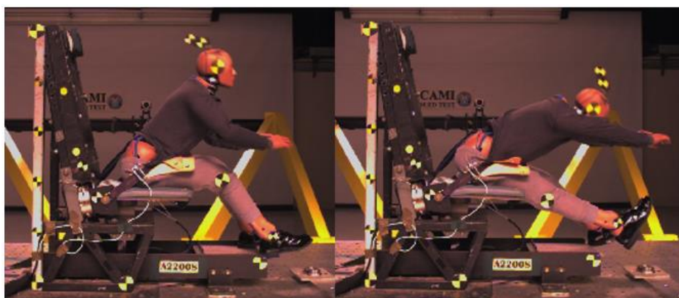
Figure 60: A22008 Picture of Peak Floor Load at 137 ms (Left) and Last Frame with Feet Touching Floor Pan at 158 ms (Right).
