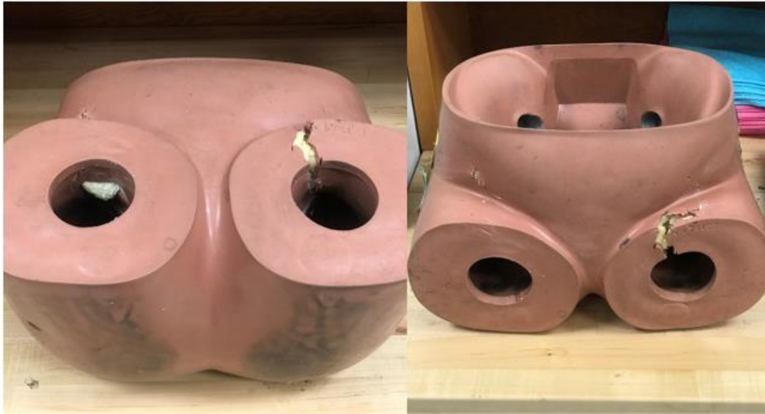
Figure 64: Damage to Pelvis at Completion of Testing.
