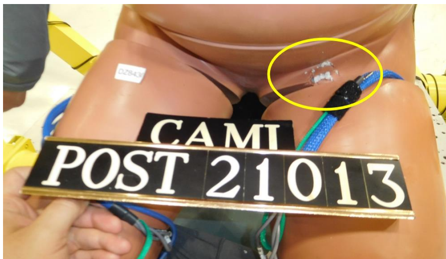
Figure 63: ATD Pelvis Damage from Belt Buckle after Seven Longitudinal Tests.
