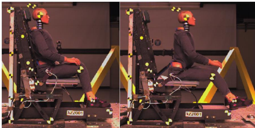
Figure 29: A22001 Peak Load Floor Load at 51 ms (Left) and Last Frame at 115 ms (Right).
