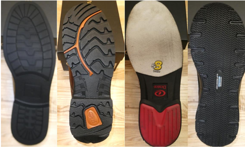
Figure 3: Footwear Tread Patterns (Left to Right): Mil Spec, Boots, Bowling Shoe, and Sneakers.
