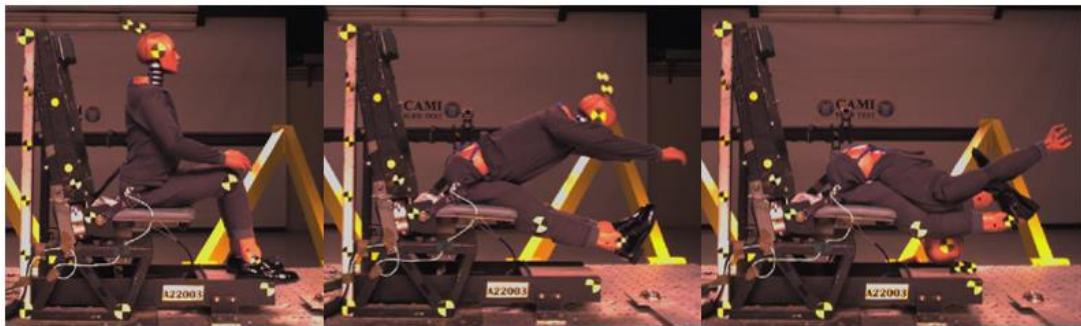
Figure 10: ATD Position at 110 (Left), 160 (Center) and 220 ms (Right), A22003.
