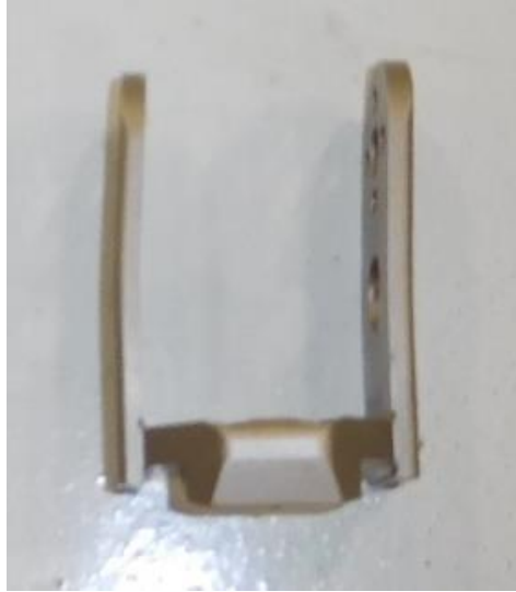
Figure 14: Bent Knee Bracket at Completion of A21015.
