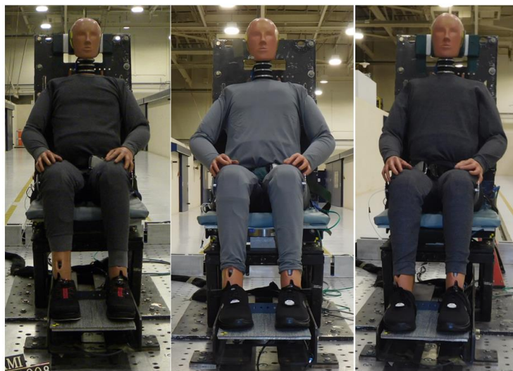
Figure 4: Tested Clothing (Left to Right): 100% Cotton, 60% Cotton/40% Polyester, and 92% Polyester/8% Spandex.
