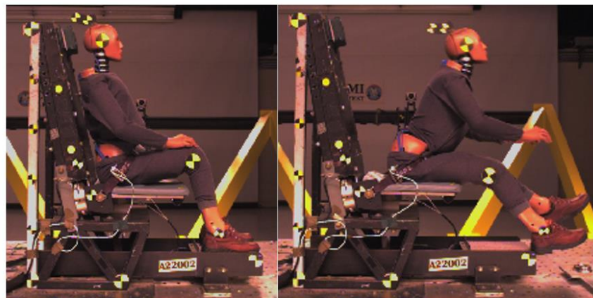
Figure 23: A22002 (Boots) Peak Load Floor-Pan Load at 62 ms (Left) and Last Frame at 130 ms (Right).
