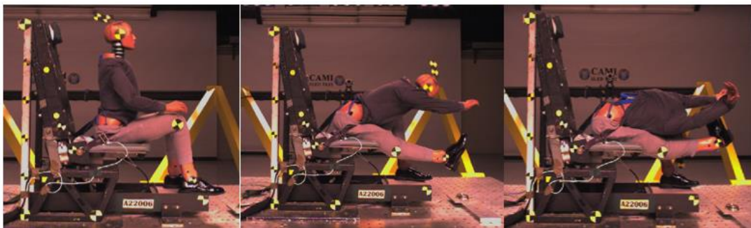
Figure 11: ATD Position at 110 (Left), 160 (Center) and 200 ms (Right), A22006.
