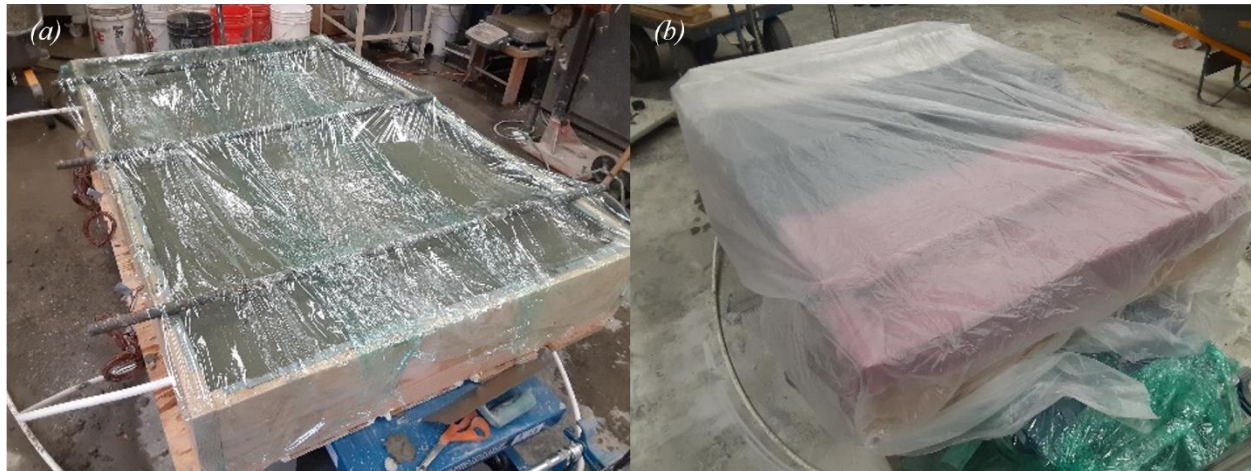
Figure 104. a) Initial 24-hour set and b) 28-day damp towel cure
