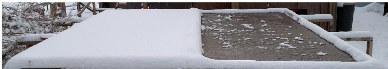
Figure 40. Photo of the deck model surface during the storm. Heat exchanger pipes have spacing of 30 cm and 20 cm in left-side and right-side model deck, respectively (Bowers Jr, 2016).
