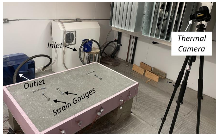
Figure 106. Bridge deck model prepared for testing
