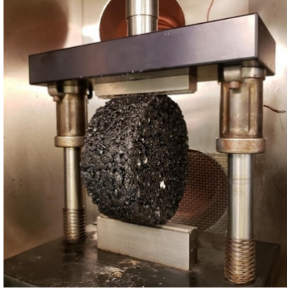
Figure 2. Photo. Test setup for IDEAL-CT.
