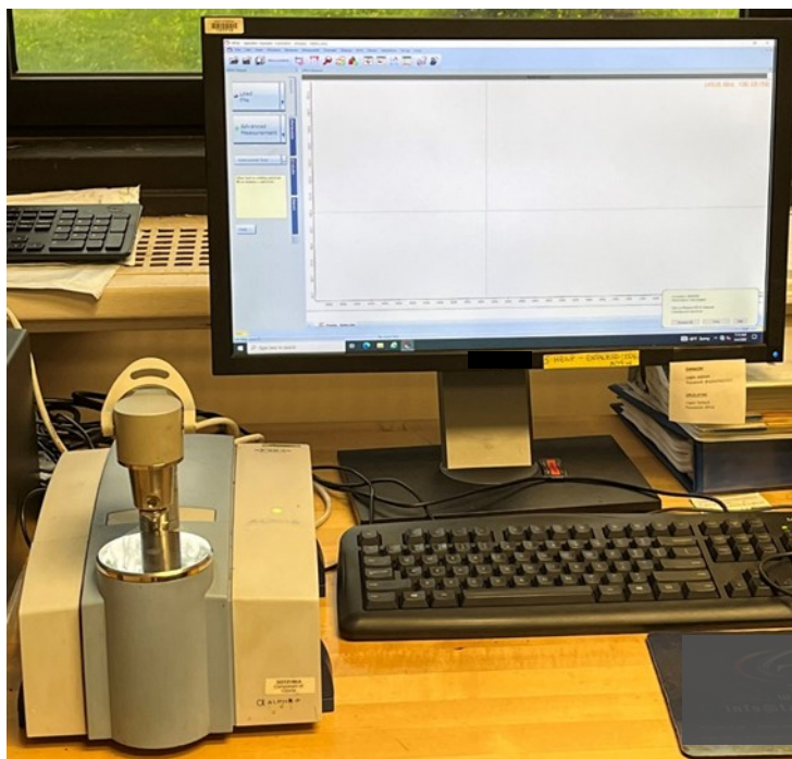
Figure 9. Photo. A Fourier transform infrared spectrometer with attenuated total reflectance capability.
