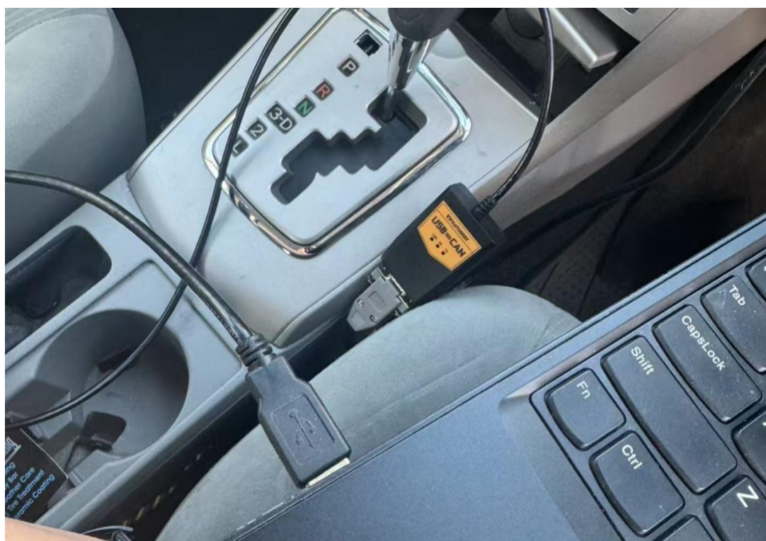
Figure 16. CAN2USB device in the probe vehicle.
