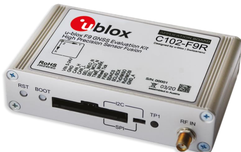
Figure 15. UBlox F9R GPS in the probe vehicle.
