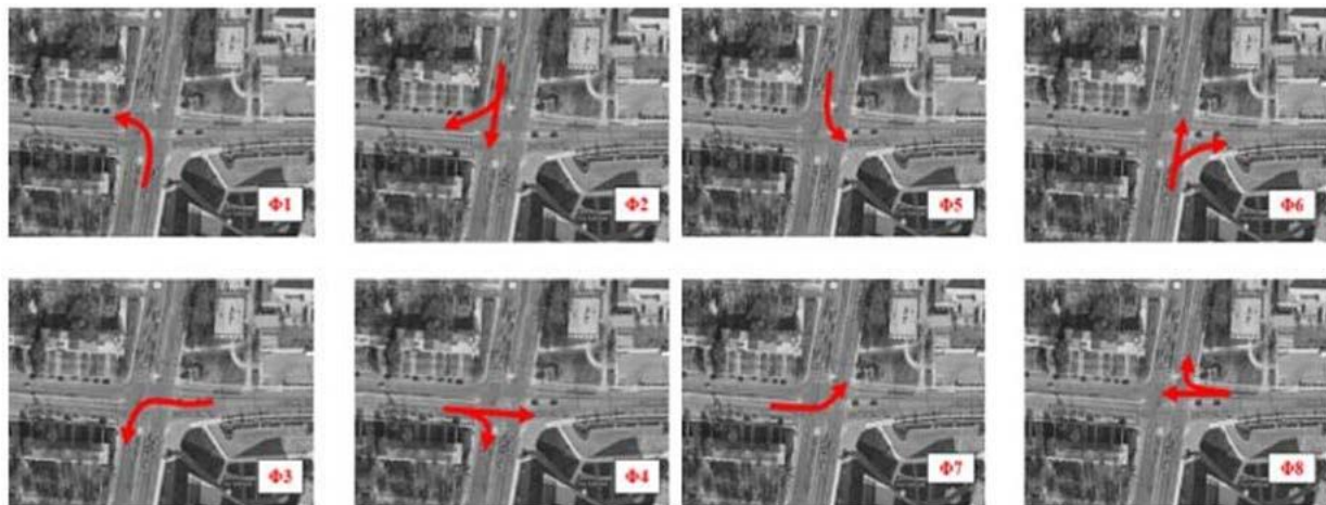
Figure 18 Different Phases of The Traffic Signal
