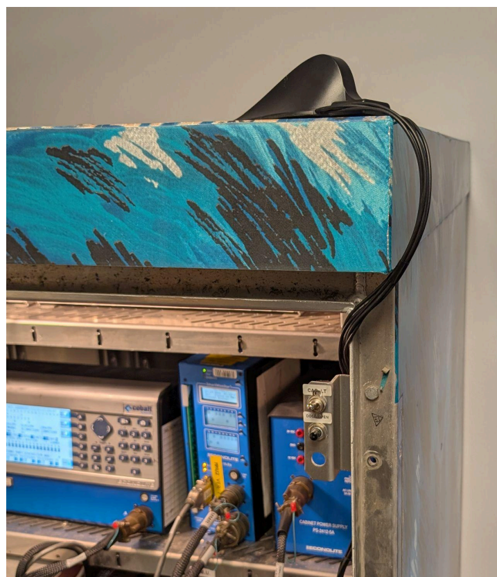
V2X antenna placement (lab environment shown)
