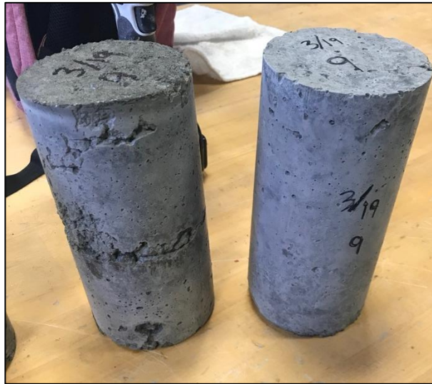
Figure 3.1 Worst (Left) and Best (Right) Compacted Cylinders Made from SF1a.
