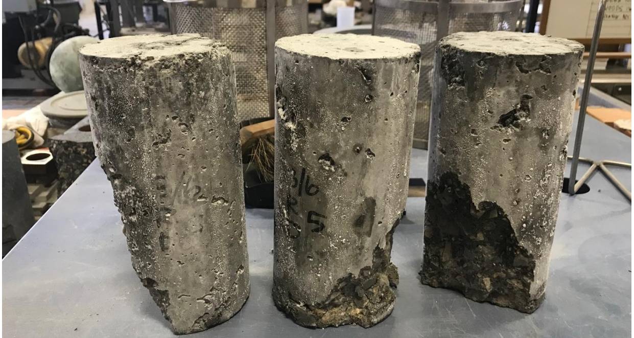
Figure E.2 Trial 5 - 7.4% Silica Fume, 15% Delta Fly Ash - Broken Cylinders after 28-Day Compression Strength Test.
