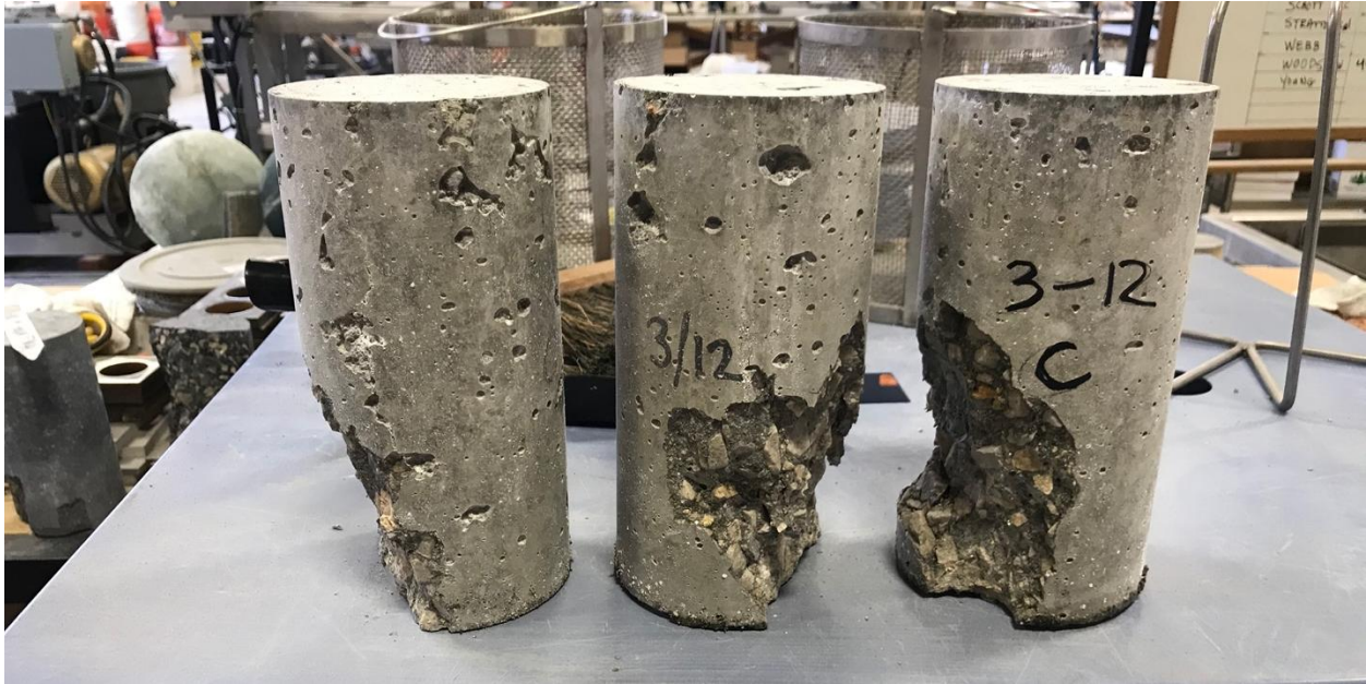
Figure E.4 Control – No SCM – Broken Cylinders after 28-Day Compression Strength Test.
