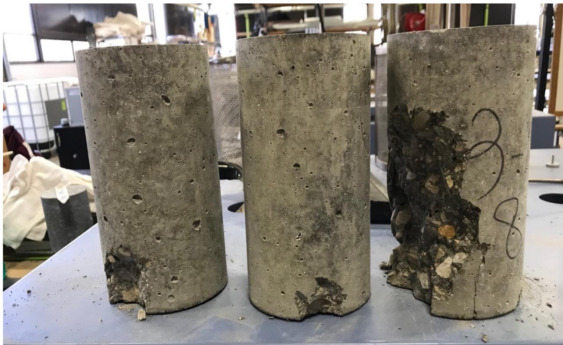
Figure E.7 Trial 8 – 15% Prairie States Fly Ash – Broken Cylinders after 7-Day Compression Strength Test.
