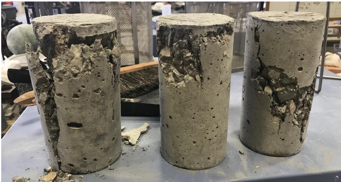
Figure E.11 Trial 10 – 15% Pumice – Broken Cylinders at 7-Day Compression Strength Test.
