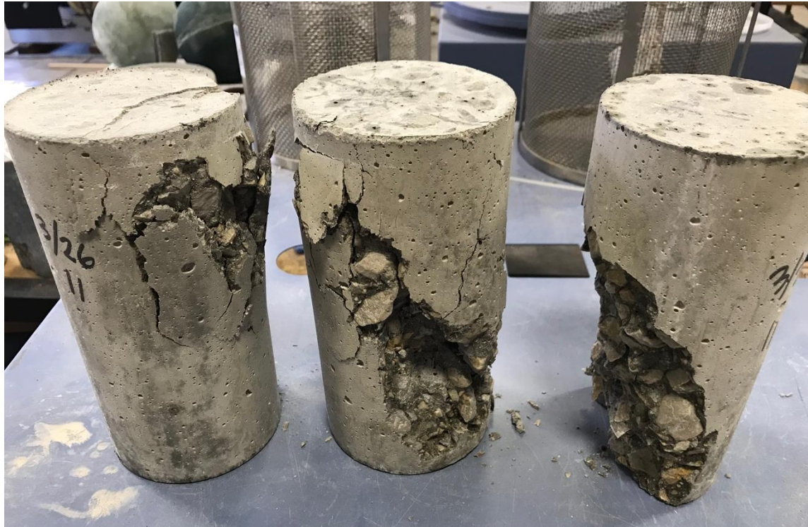
Figure E.14 Trial 11 – 15% Waste Glass Powder – Broken Cylinders after 28-Day Compression Strength Test.
