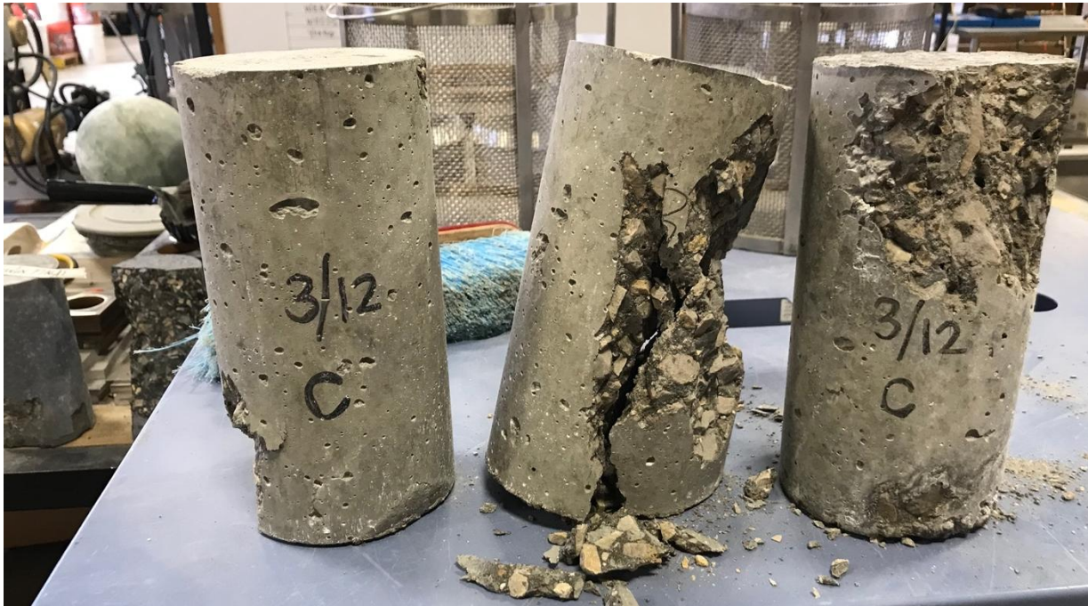
Figure E.3 Control – No SCM - Broken Cylinders after 7-Day Compression Strength Test.
