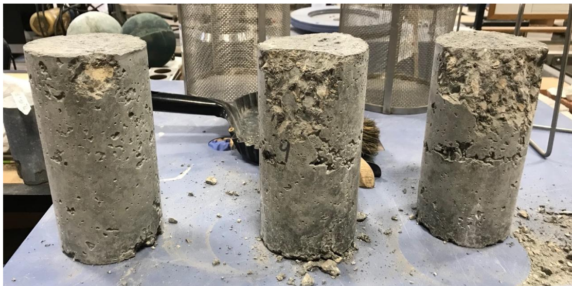
Figure E.9 Trial 9 – 9% Silica Fume – Broken Cylinders after 7-Day Compression Strength Test.
