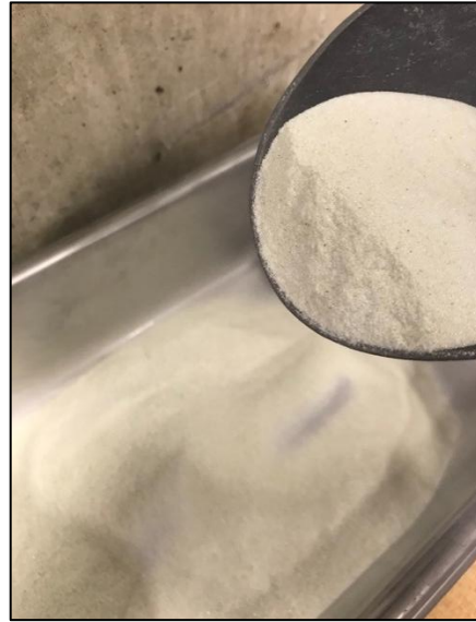
Figure 2.1 Waste Glass Powder Sample Collected from Momentum Recycling's Air Filtration System.
