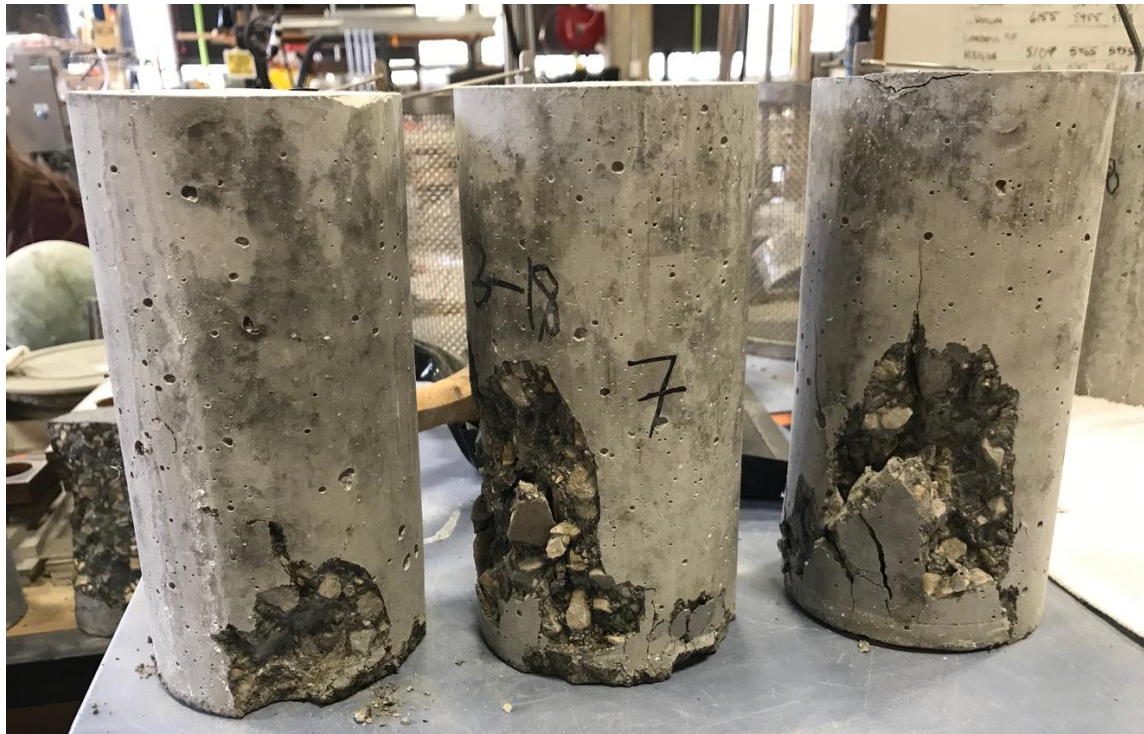
Figure E.6 Trial 7 – 15% Delta Fly Ash – Broken Cylinders after 28-Day Compression Strength Test.
