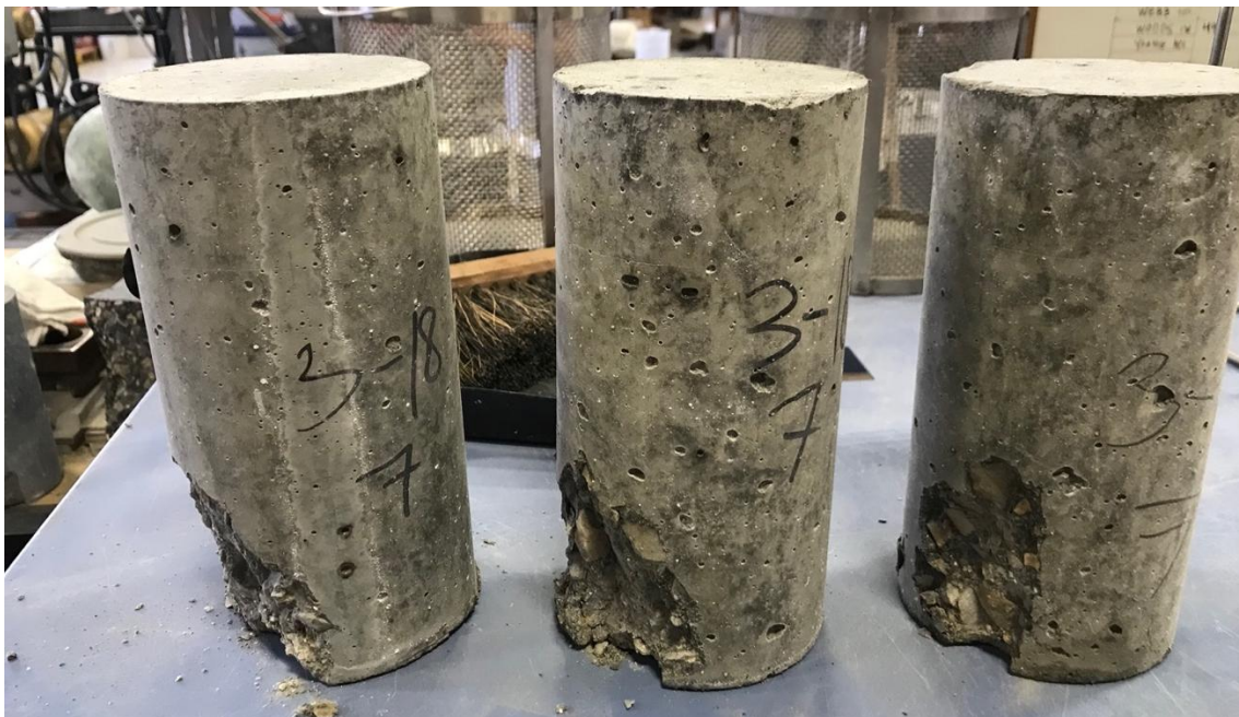
Figure E.5 Trial 7 – 15% Delta Fly Ash – Broken Cylinders after 7-Day Compression Strength Test.
