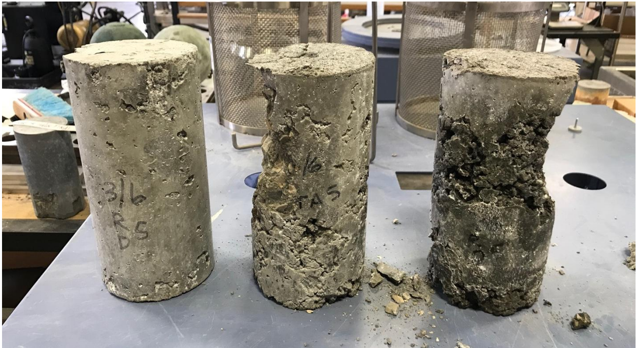
Figure E.1 Trial 5 - 7.4% Silica Fume, 15% Delta Fly Ash - Broken Cylinders after 7-Day Compression Strength Test.
