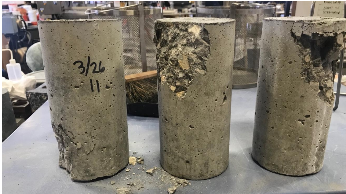
Figure E.13 Trial 11 – 15% Waste Glass Powder – Broken Cylinders after 7-Day Compression Strength Test.
