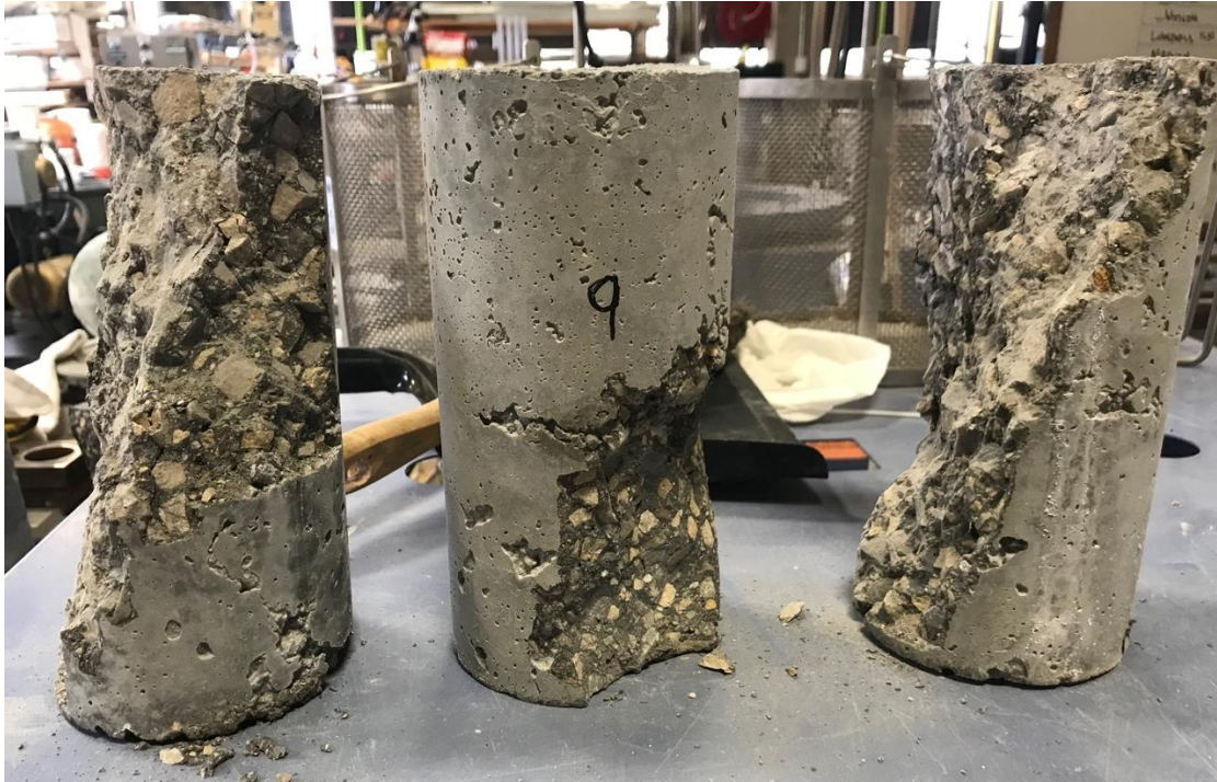
Figure E.10 Trial 9 – 9% Silica Fume – Broken Cylinders after 28-Day Compression Strength Test.
