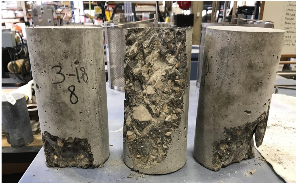
Figure E.8 Trial 8 – 15% Prairie States Fly Ash – Broken Cylinders after 28-Day Compression Strength Test.
