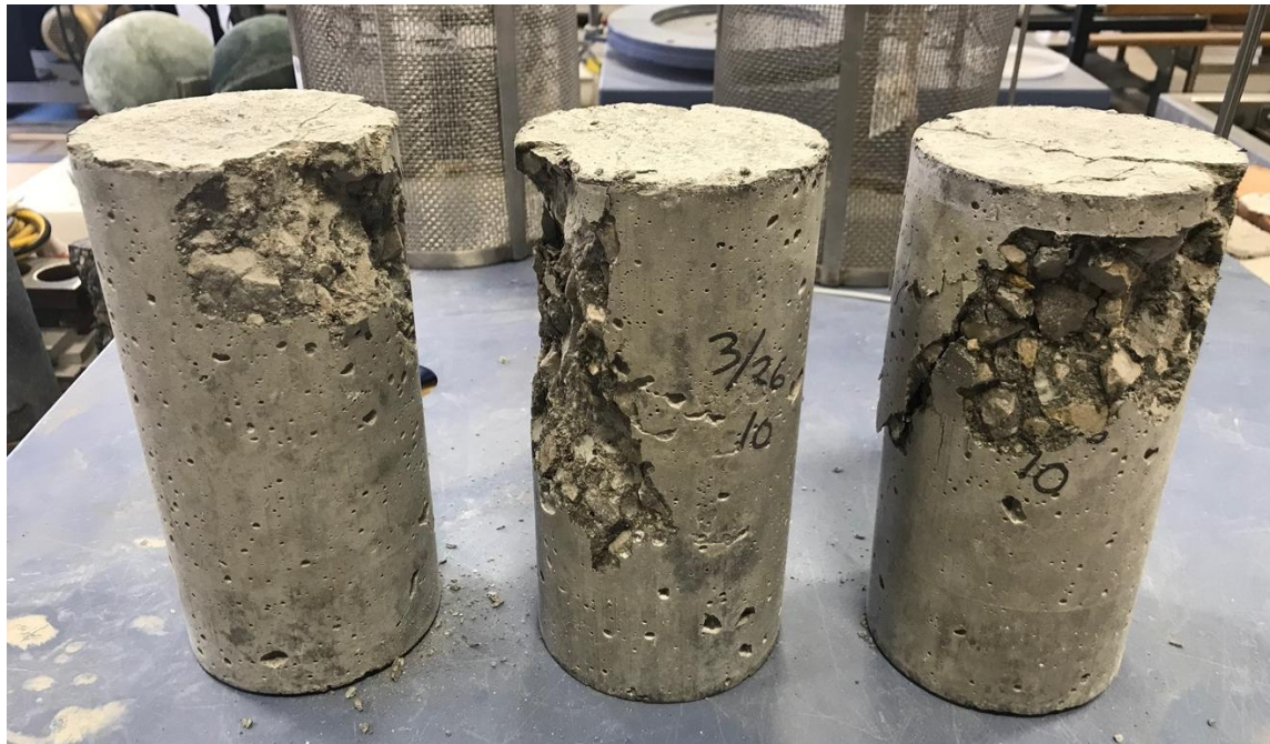
Figure E.12 Trial 10 – 15% Pumice – Broken Cylinders at 28-Day Compression Strength Test.
