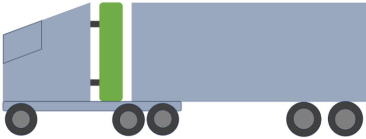
Figure 3. Proposed BET design for easy battery swapping.
