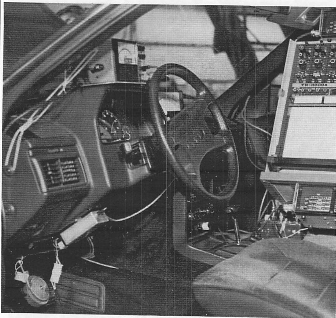
Figure E-2: Modified cruise control is shown mounted just below dash board. The brake pedal force transducer reading is displayed on the large meter above the speedometer.
