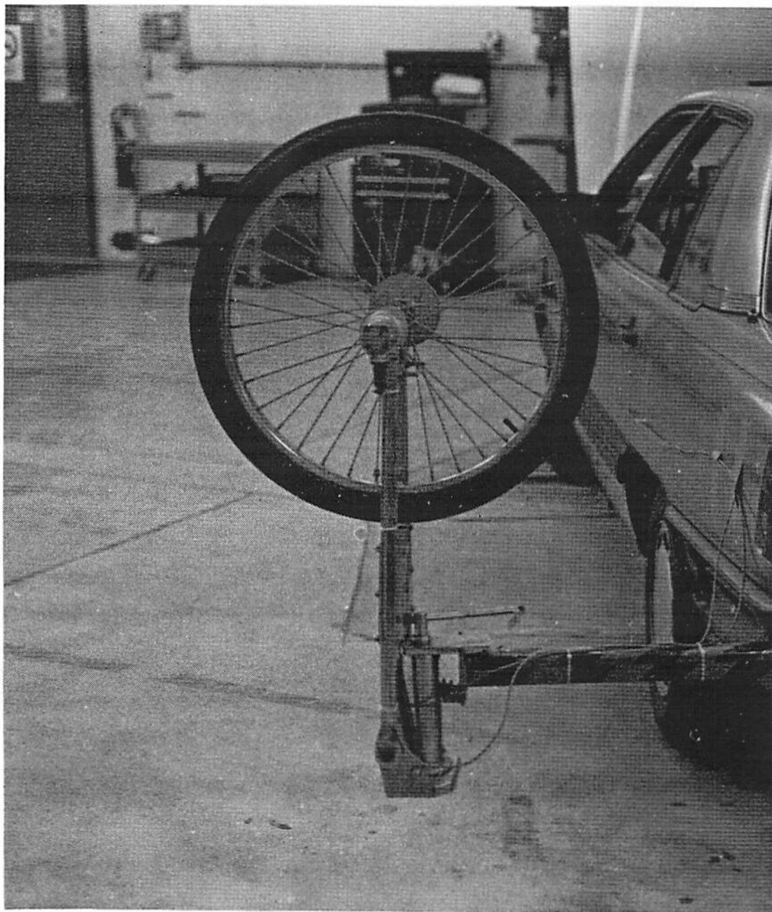
Figure E-3: The fifth wheel is pivoted at the side so that it can readily be used in both forward and reverse.
