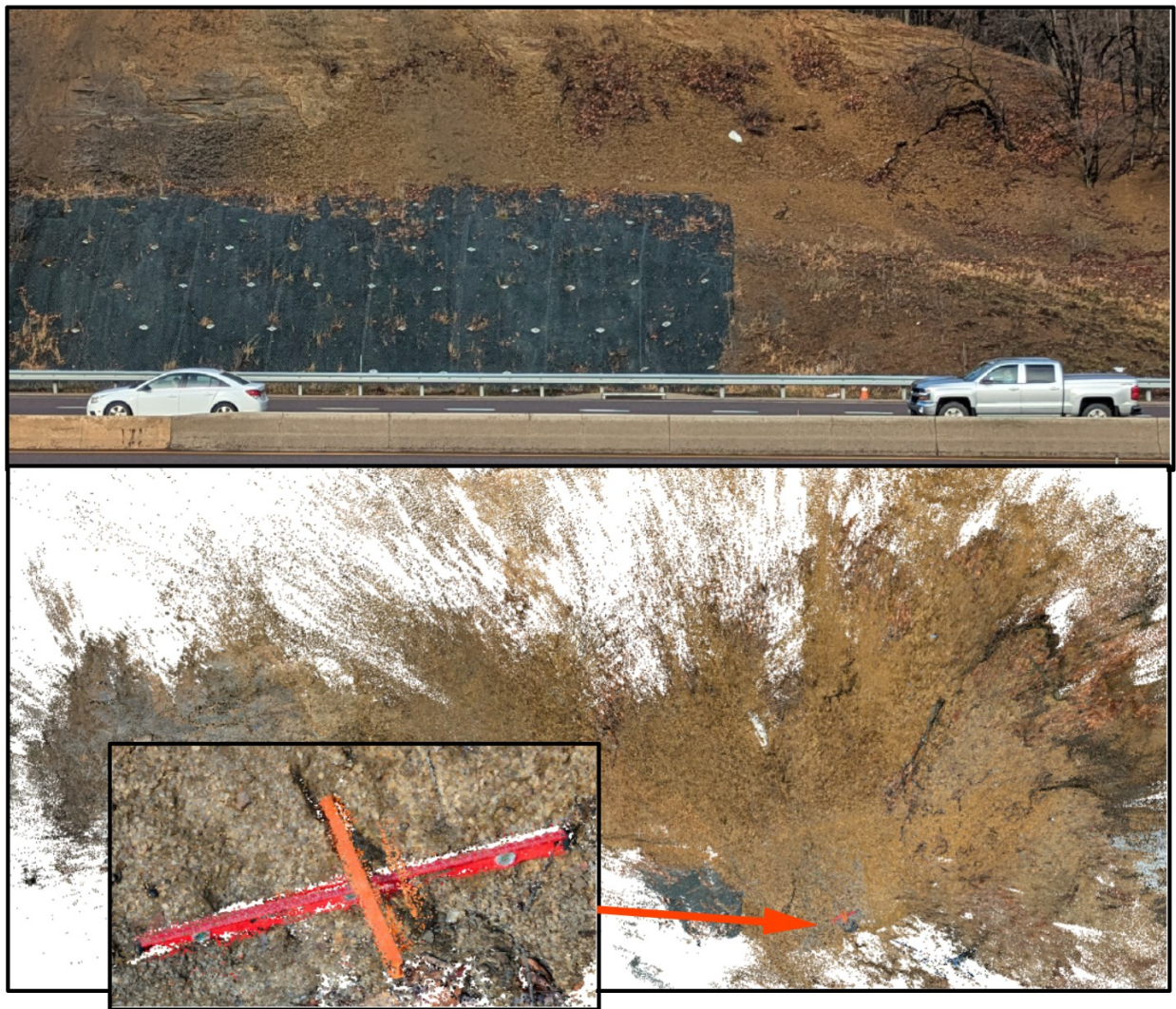
Figure 3: 3D reconstruction (bottom) of a hill side (top). The insert shows the 3D point cloud of the levels. Notice that the orange level has a faint double. This is a sign of misalignment.
