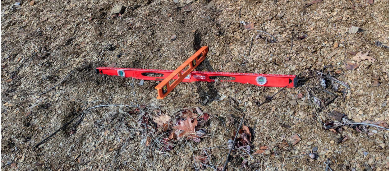
Figure 2: Two levels that will allow the 3D reconstruction to be scaled and leveled.
