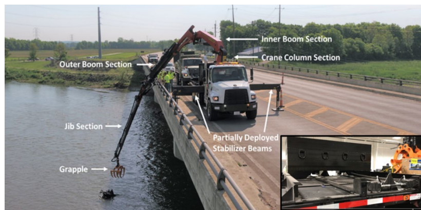
Figure 1: Knuckleboom crane with safety software to prevent overloading when outriggers cannot be fully deployed. The inset picture in the lower right shows the custom 12,000-lb counterweight system that shifts away from the working side of the crane to offset impact of partially deployed outriggers to maintain lifting capacity of the crane.
