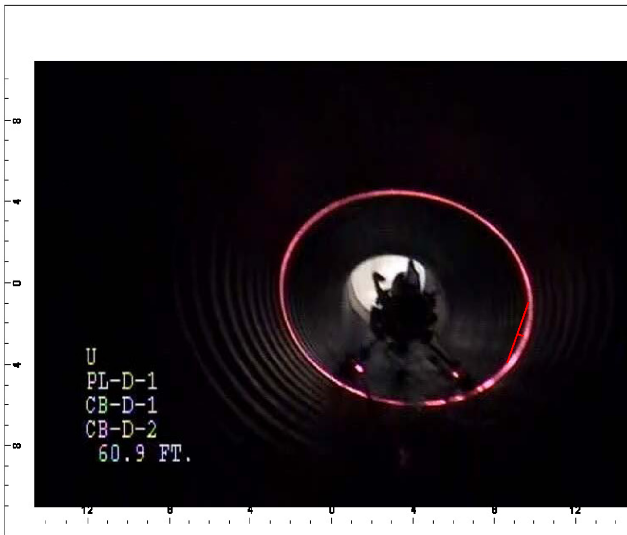
Figure 25 - Laser ring profiler with chord and sagitta
