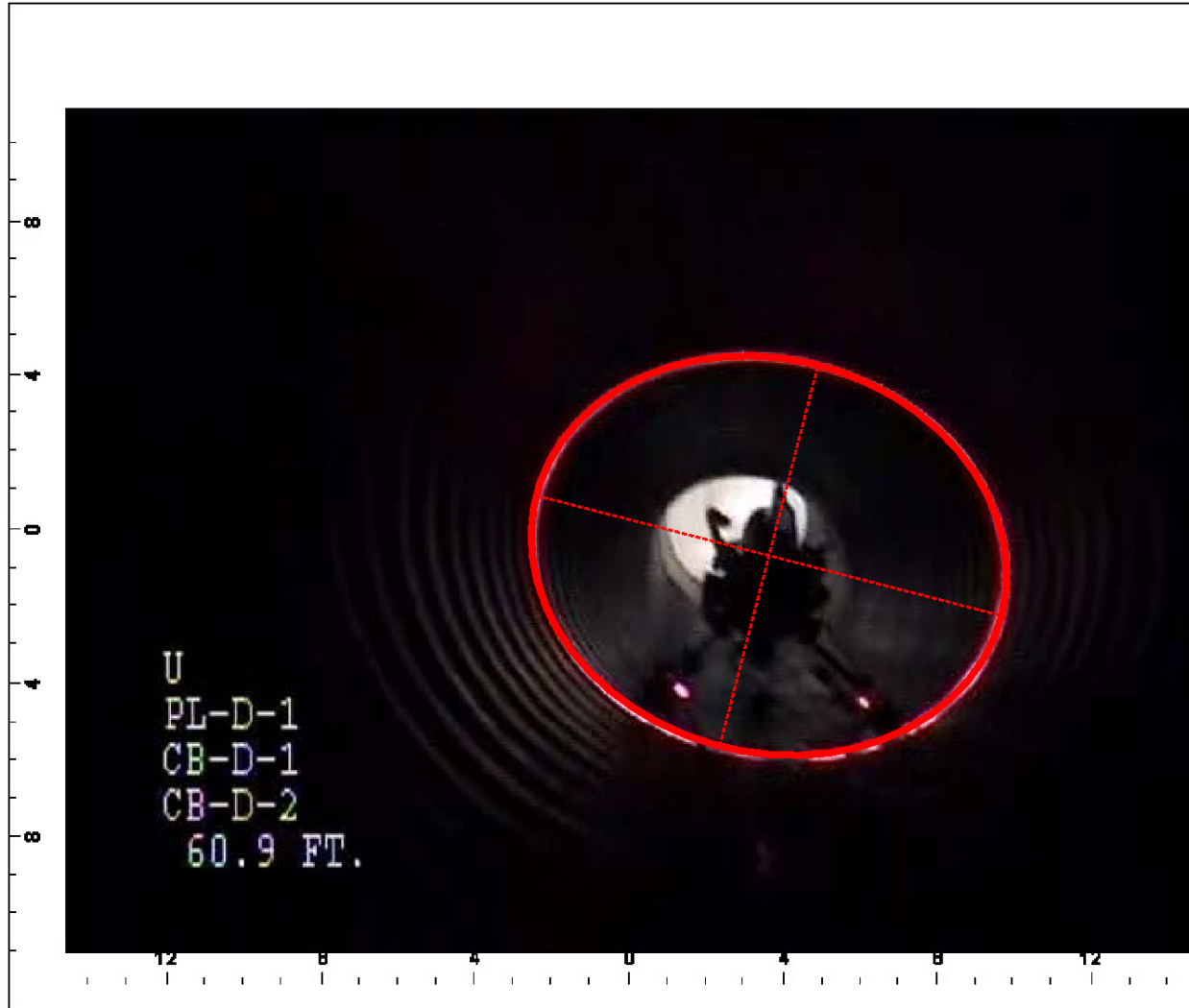
Figure 24 - Laser ring profiler with superimposed best-fit ellipse
