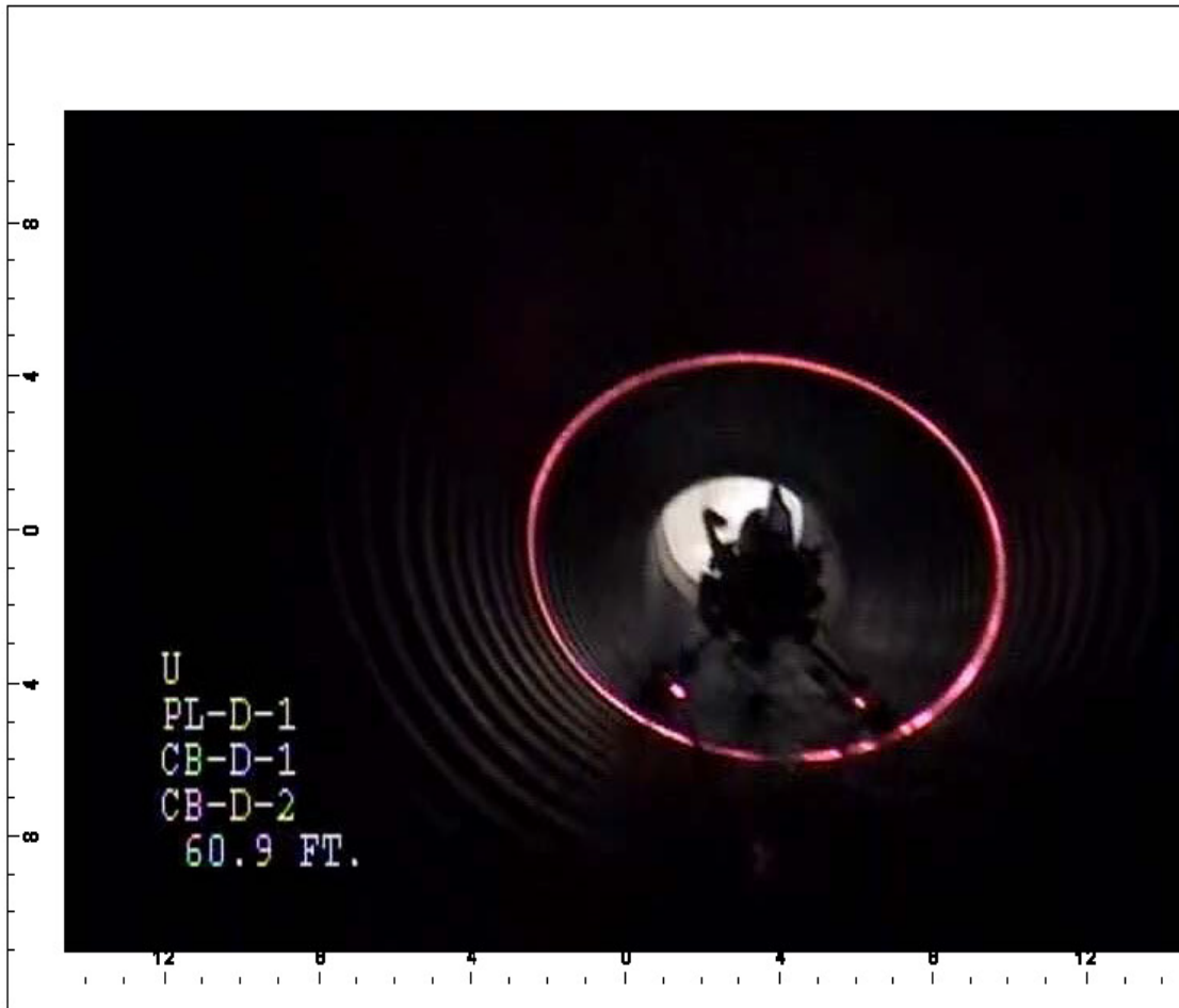
Figure 23 - Laser ring profiler cross-section
