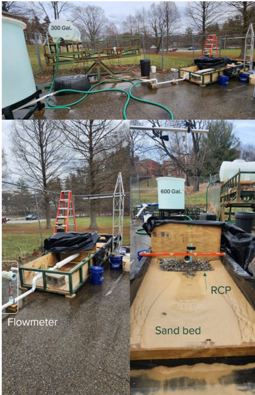
Figure 5 Experimental Setup of Physically Scaled RCP in Hydraulic Flume at Ohio University (1 gal = 3.79 l)
