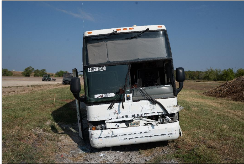
Figure 12.3. Front of Test Vehicle after Test 440213-01-6.
