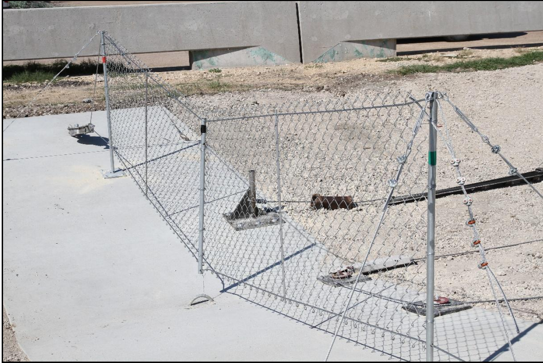
Figure 4.5. First Median Opening Protection System prior to Crash Tests 440210-01-1&2.
