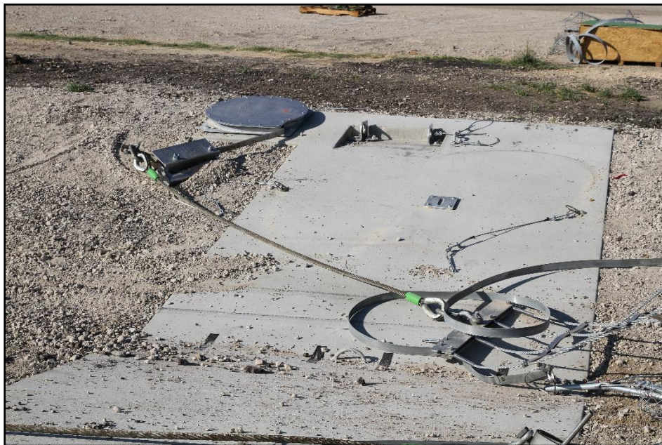
Figure 8.6. Second Net Swivel Anchor and Energy Absorbers after Test 440210-01-2.
