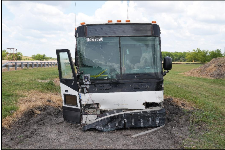
Figure 11.3. Front of Test Vehicle after Test 440211-01-5.
