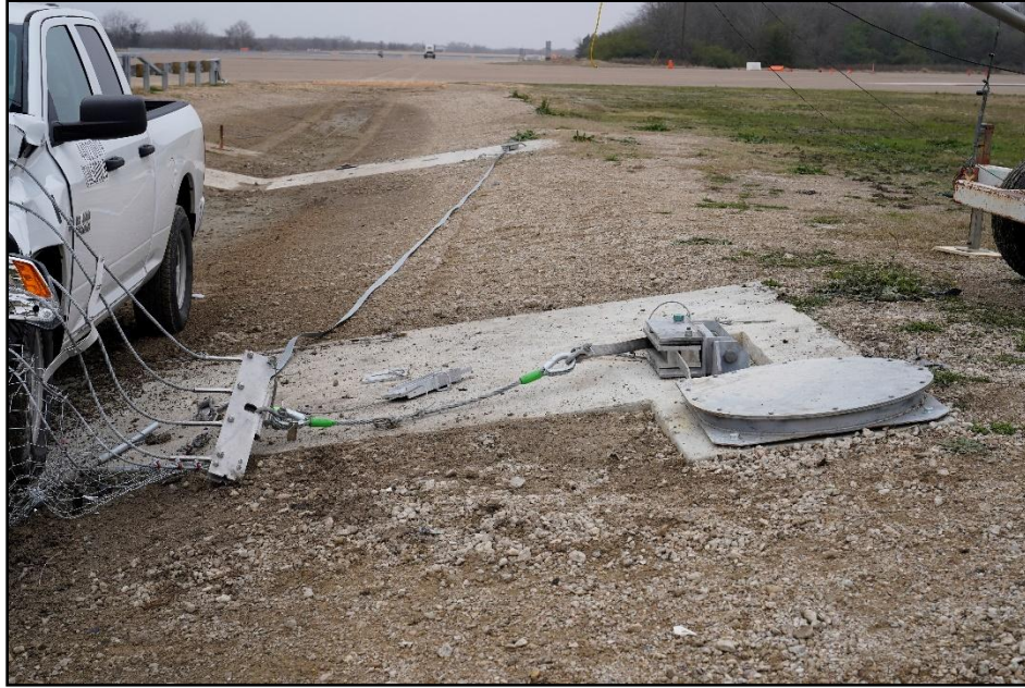
Figure 9.6. Second Net Swivel Anchor and Energy Absorbers after Test 440210-01-4.
