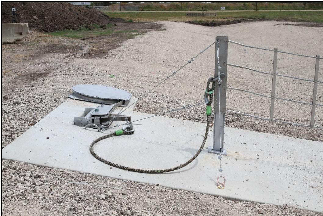
Figure 4.8. Anchor Hardware for the Second Median Opening Protection System Net prior to Crash Tests 440210-01-1&2.
