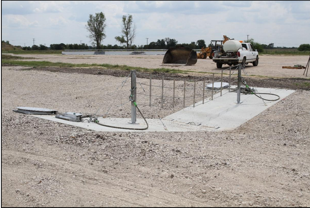
Figure 4.7. Second Median Opening Protection System Net prior to Crash Tests 440210-01-1&2.
