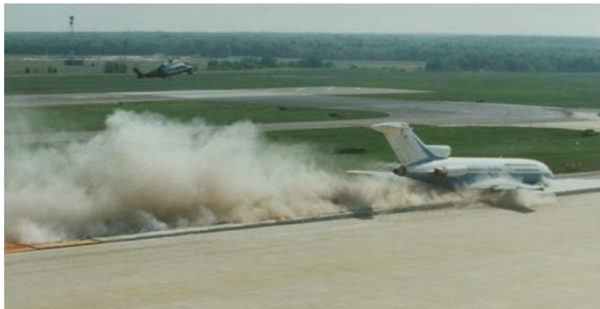
Figure 3.3. EMAS Airplane Test (5).
