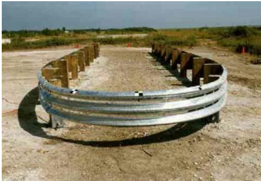
Figure 3.5. MwRSF Bullnose System (7).
