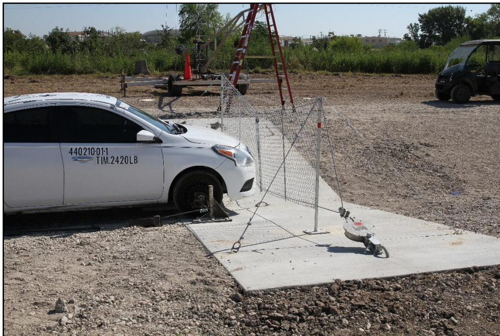
Figure 7.2. MOPS/Test Vehicle Impact Location for Test 440210-01-1.
