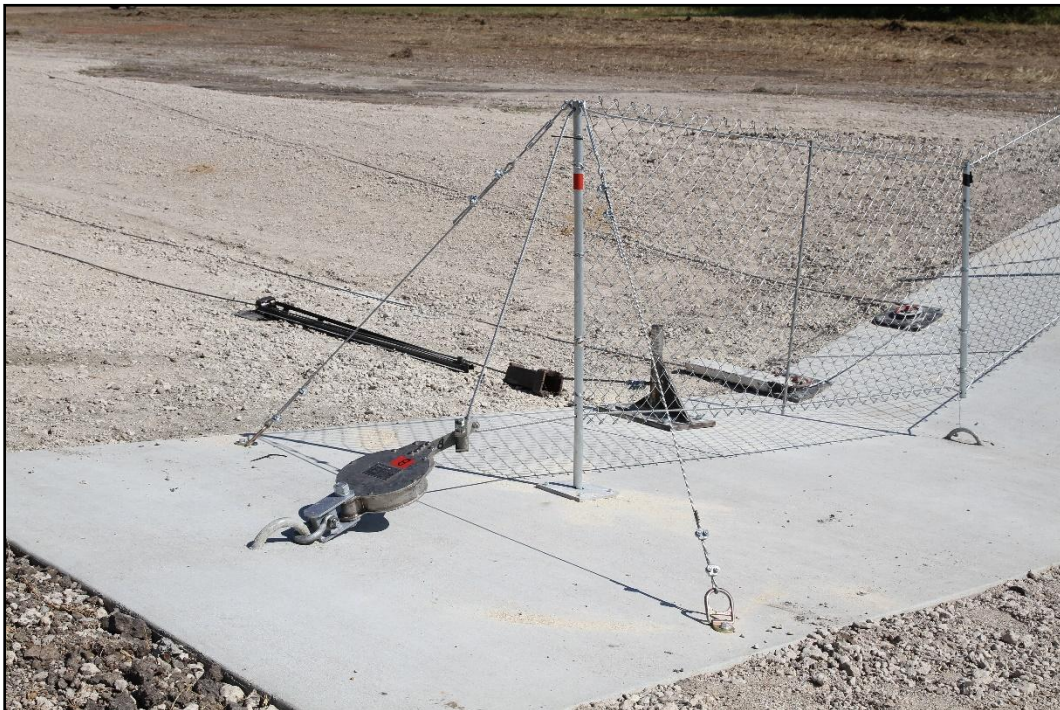
Figure 4.6. Anchor Hardware for the First Median Opening Protection System prior to Crash Tests 440210-01-1&2.
