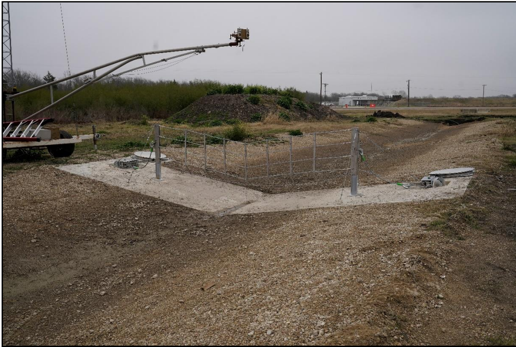
Figure 4.10. Second Median Opening Protection System Net prior to Crash Tests 440210-01-4, 440211-01-3, 440211-01-5, and 440213-01-6.
