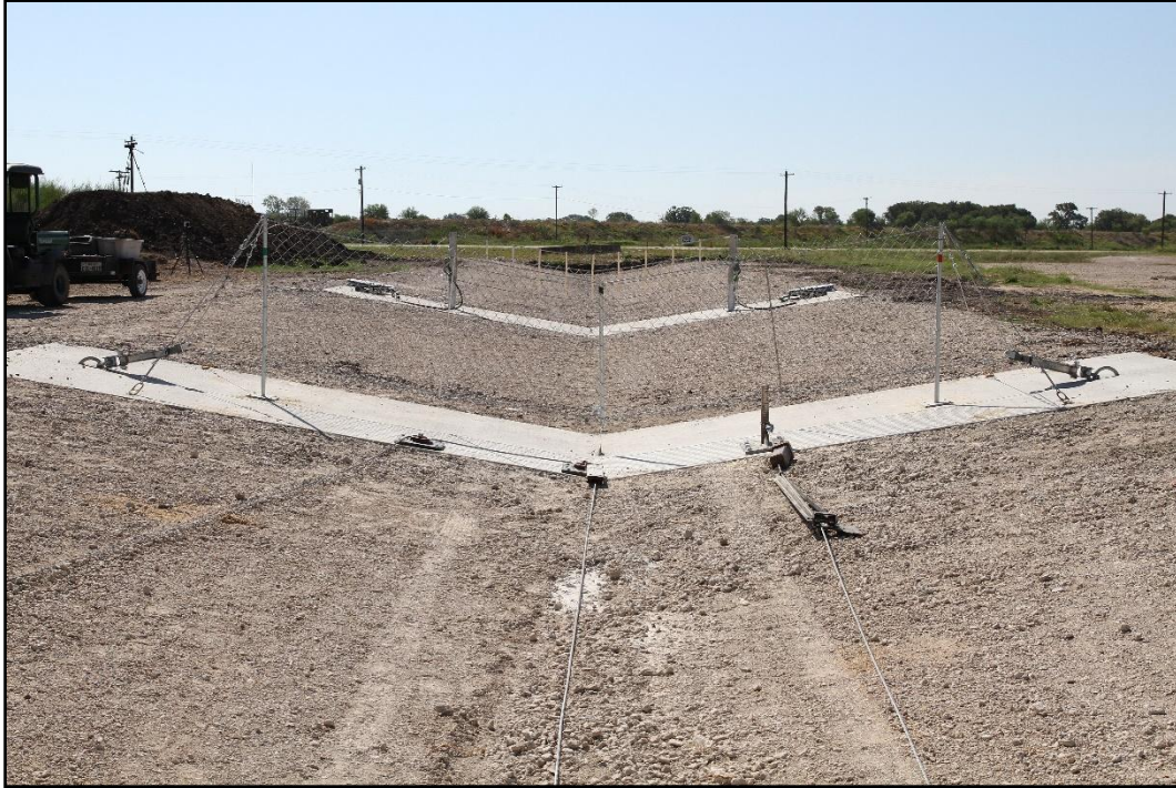
Figure 4.3. Upstream In-Line View of the Median Opening Protection System prior to Crash Tests 440210-01-1&2.
