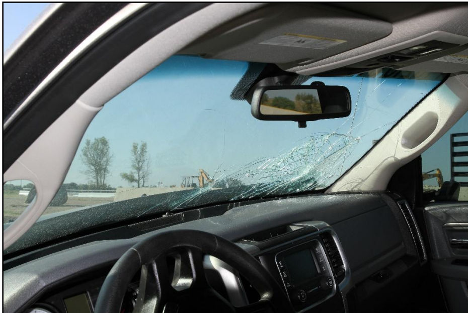
Figure 8.10. Upper Interior of Test Vehicle after Test 440210-01-2.
