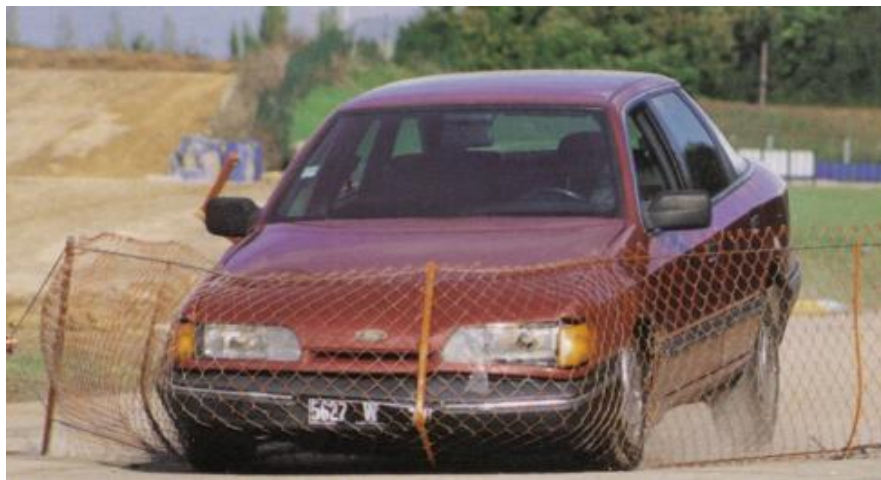
Figure 3.8. Vehicle Arresting Net (3).
