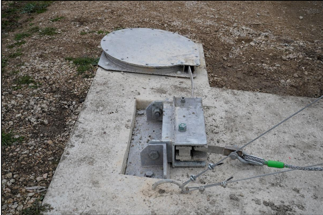
Figure 4.13. Swivel Mound System and Cannister for the Second Net prior to Crash Tests 440210-01-4, 440211-01-3, 440211-01-5, and 440213-01-6.
