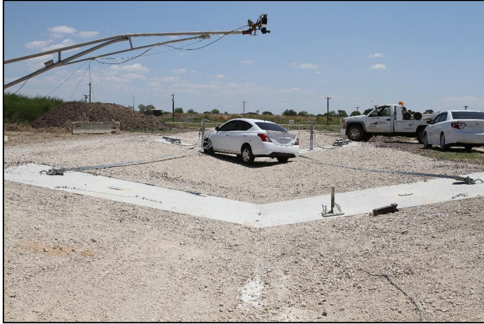
Figure 7.5. MOPS after Test 440210-01-1.
