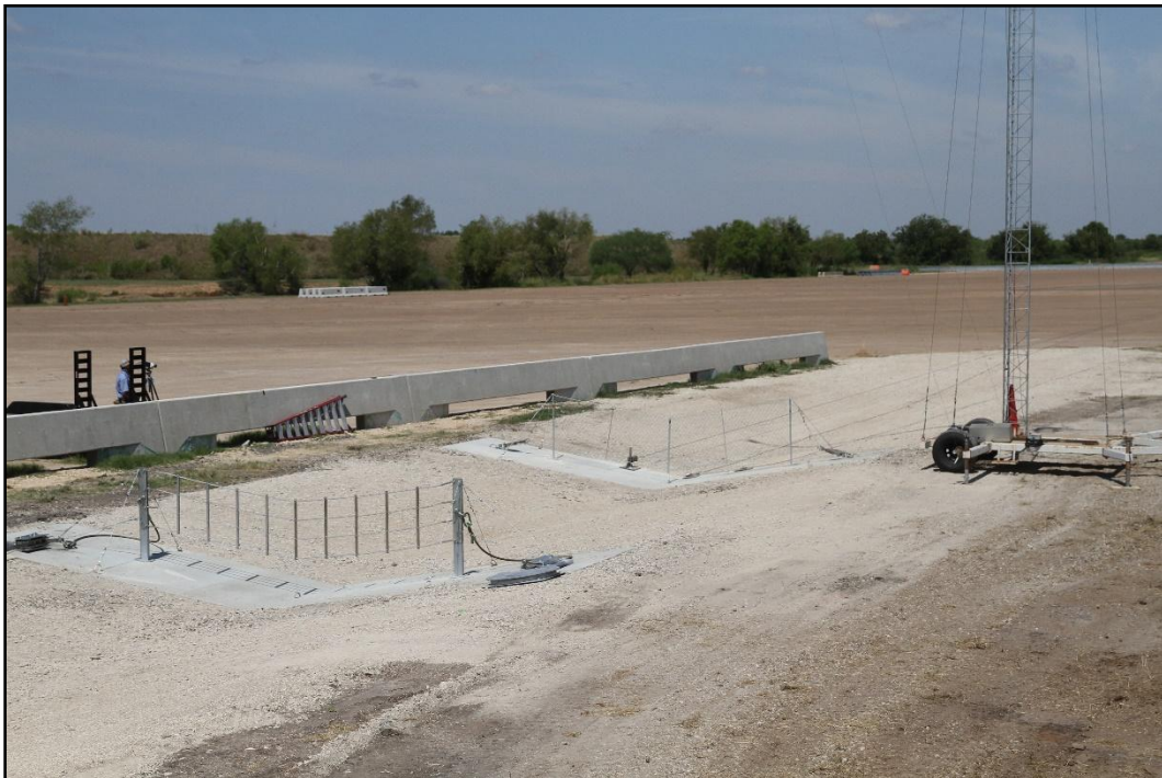
Figure 4.4. Oblique View of the Median Opening Protection System prior to Crash Tests 440210-01-1&2.
