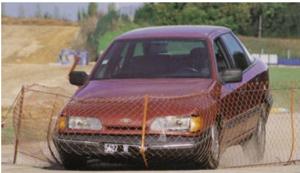
Figure 3.1. Vehicle Arresting Net (3).
