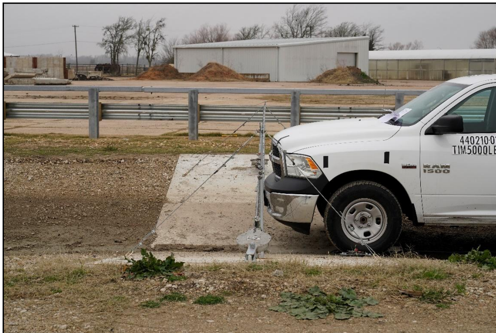
Figure 9.2. MOPS/Test Vehicle Impact Location for Test 440210-01-4.
