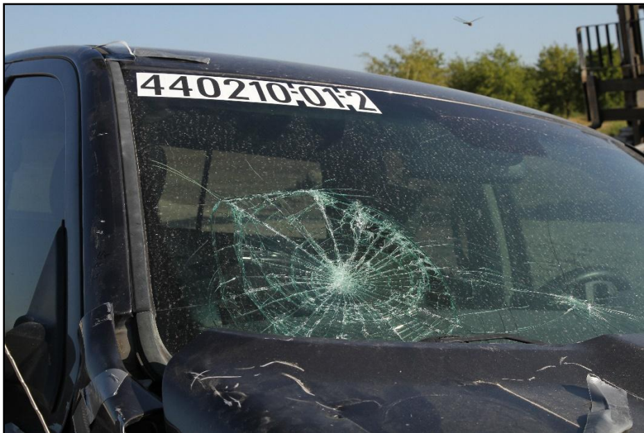
Figure 8.8. Windshield of Test Vehicle after Test 440210-01-2.
