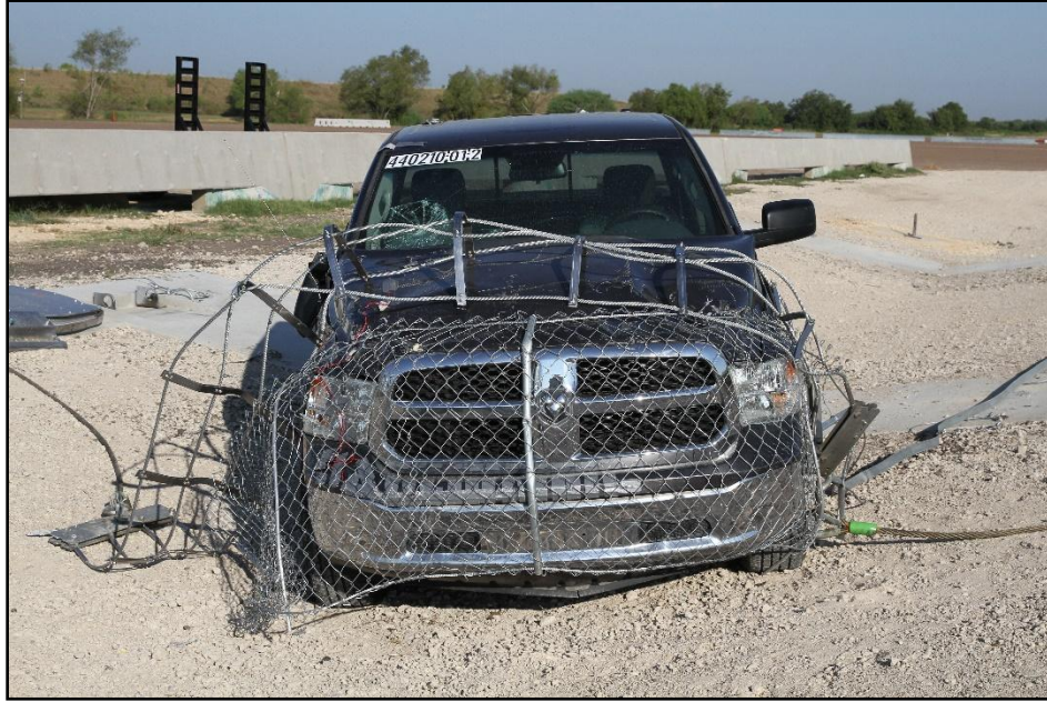
Figure 8.5. MOPSSs after Test 440210-01-2.
