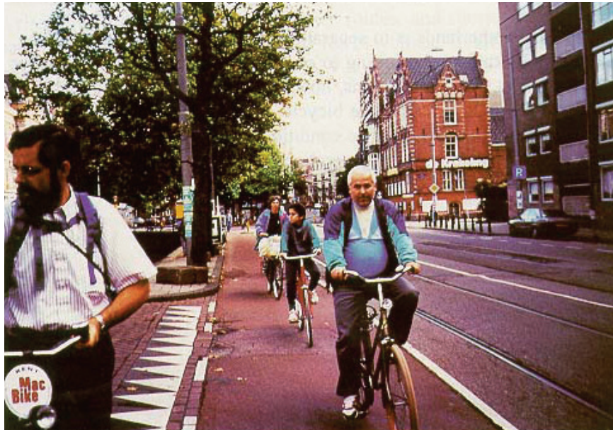
Figure 23-10. Typical bicycle lanes in The Netherlands have red pavement color and are wide enough for two bicyclists.
