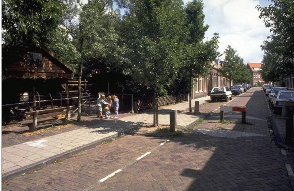
Figure 20-13. Photo. The design of street closures should provide specific parking areas to discourage obstruction of bicycle and pedestrian traffic.
