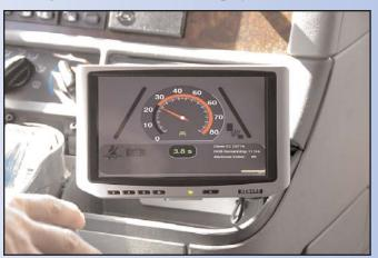
remains constant. Also, beneath the green vehicle icon is the car following gap, given in seconds. Finally, the "driver ID", "HOS [hours of service] remaining" and "Alertness Index" are also provided as direct feedback of a prototypical digital tachometer. A drowsiness/alertness warning which supplements that subsystem's COTS-based feedback is also provided.
