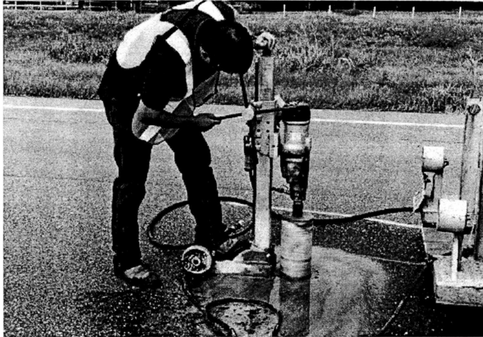
Figure 3.1 Coring of Pavement Test Section for Aggregate Extraction
