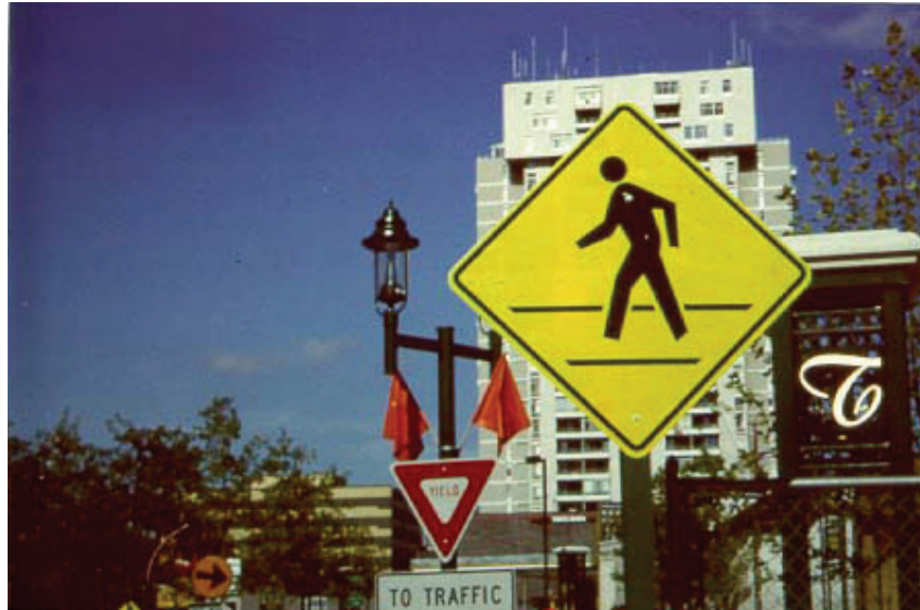
Figure 10-5. Photo. This pedestrian crossing sign is fluorescent yellow green (FYG), allowing it to be more visible.
