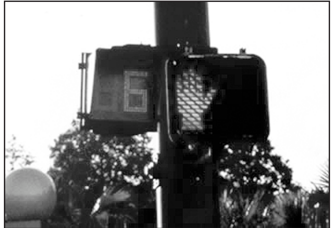
Countdown signals like the one shown above enhance safety by letting pedestrians know how many seconds they have left until the light changes.
